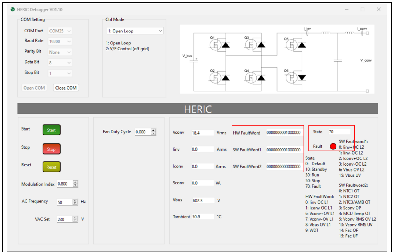
Figure 48 Fault indication in the GUI
