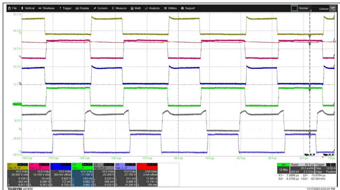
Figure 33 Switching signals for 36 V input at 12 A phase “U” current V_{GS\_HS\_W} (yellow), V_{GS\_LS\_W} (red), V_{GS\_HS\_V} (blue), V_{GS\_LS\_V} (green), V_{GS\_HS\_U} (grey), V_{GS\_LS\_U} (light blue), Phase “U” current (orange)
