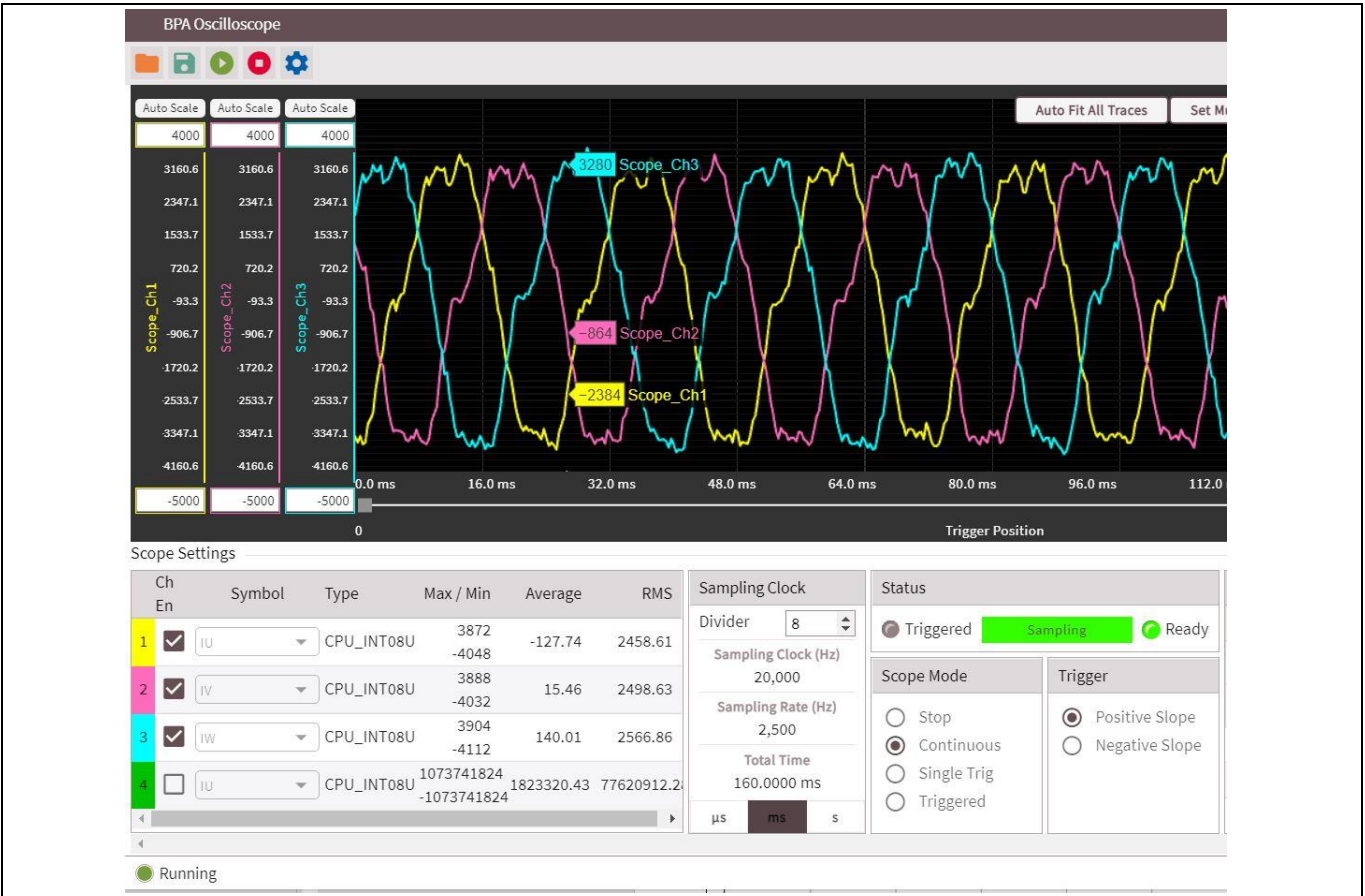
Figure 15 V/f open loop IU, IV, and IW current waveforms captured by the GUI's oscilloscope
