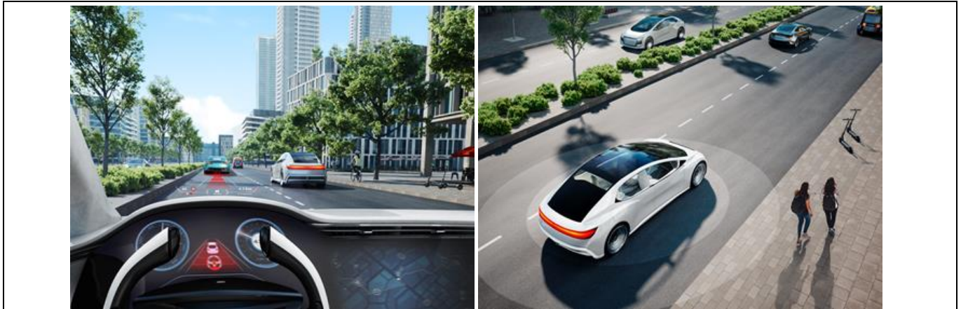
Figure 26 Artistic rendering of ADAS applications – maintaining a safe distance from the vehicle in front (left) and pedestrian detection (right)
