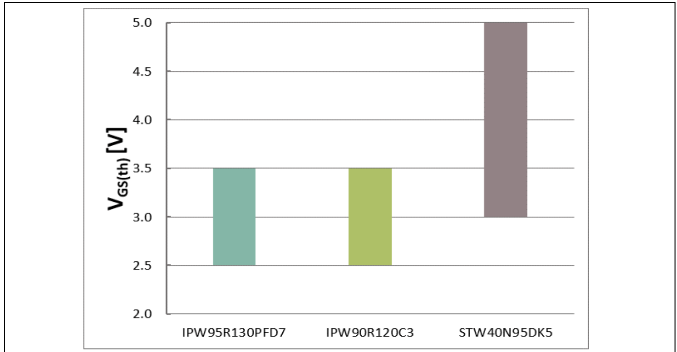
Figure 11 Low V_{GS(th)} and tight V_{GS(th)} deviation
