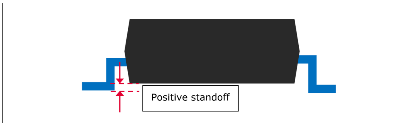
Figure 6 Positive package standoff (DDPAK + QDPAK)
