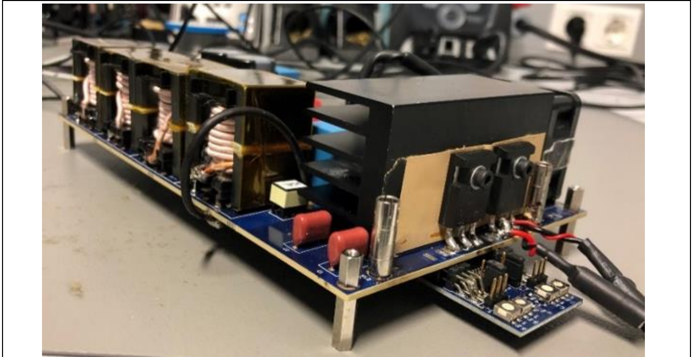
Figure 44 Heatsink design of triangular current board (equipped with standard TO-247-3)
