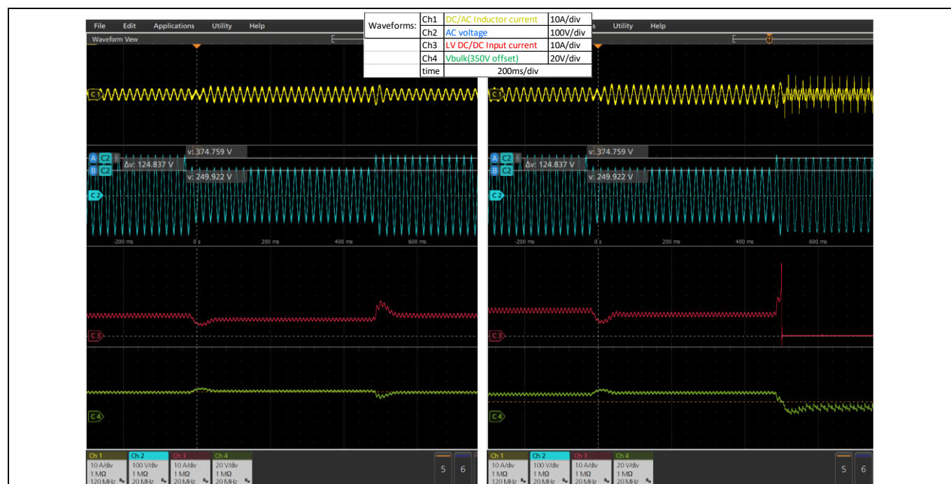
Figure 34 265 to 176 V AC voltage variation for 960 W (left) and 1200 W (right) in the inverter operation
