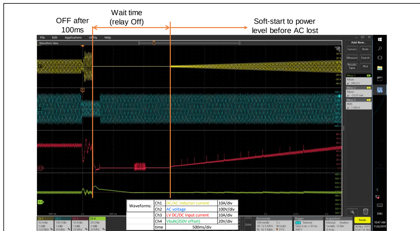
Figure 32 115 V/200 ms voltage sag from 230 V at 2.5 kW inverter operation
