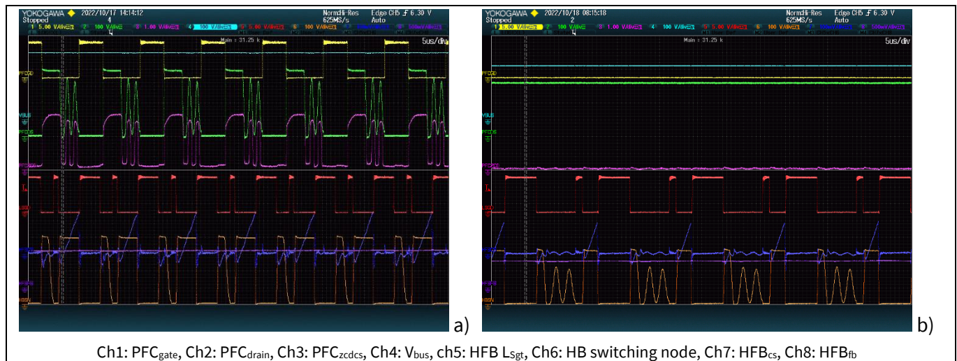
Figure 17 Continuous operation mode with HFB in ZV-RVS mode: a) PFC switching at third valley at 115 V input and 28 V 2 A output, and b) PFC disabled at 230 V, 15 V 1 A output
