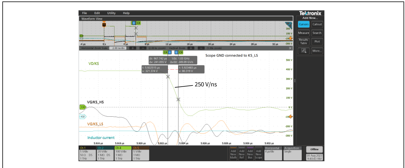
Figure 26 Maximum dV/dt achieved with hybrid configuration and proposed layout 1
