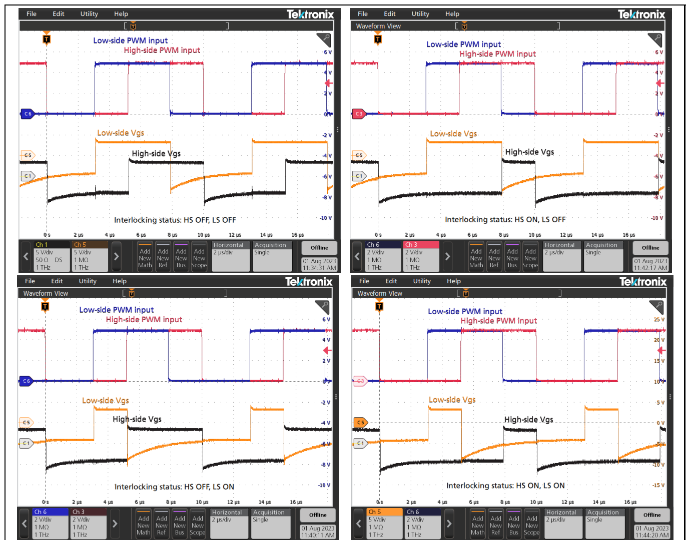
Figure 21 PWM inputs and driving voltages with different interlocking configurations
