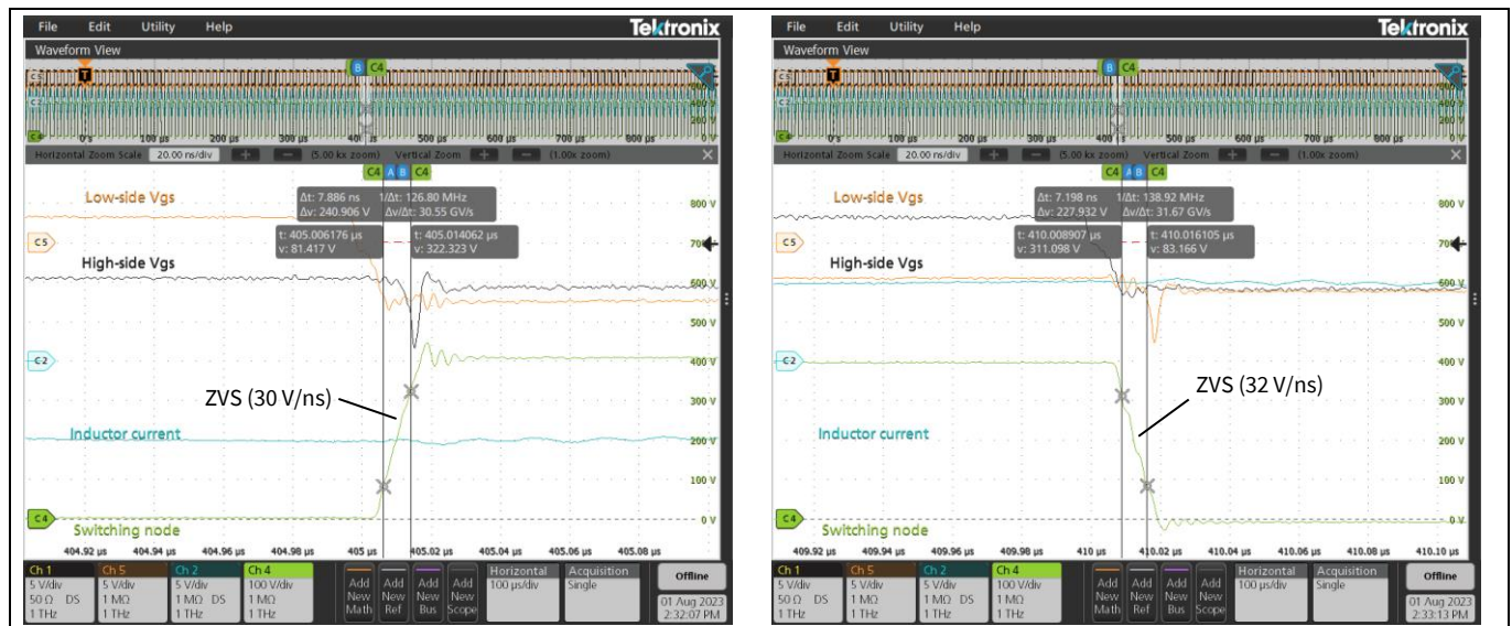
Figure 30 100 kHz soft-switching with 200 ns DT, inductive load 50 \mu H, no DC load (zoom)
