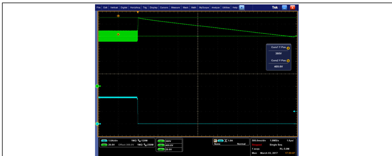
Figure 20 Load step: 100% → 0% at V_{IN} = 115 V AC
