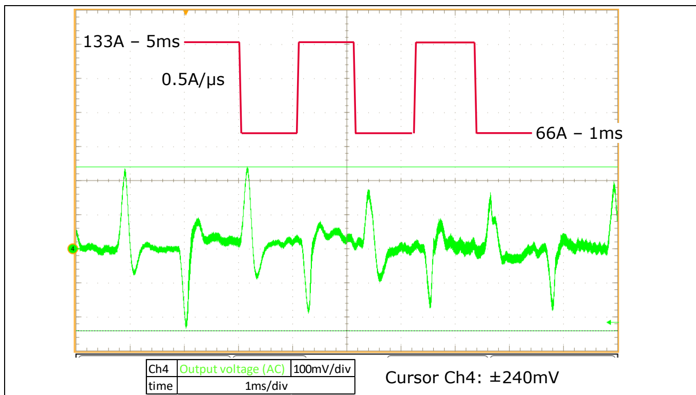
Figure 16 Output voltage response to 132 A to 66 A dynamic load steps with 0.5 A/μs current slope every 1 ms
