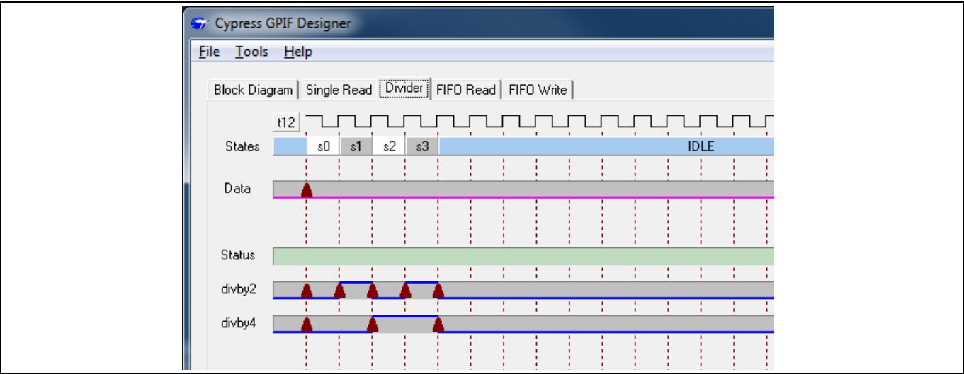
Figure 17 Div by 2 and Div by 4 Waveforms
