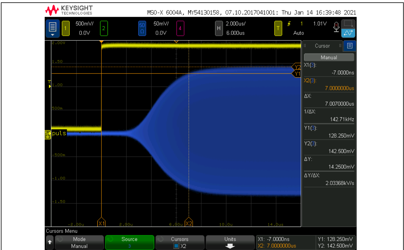
Figure 19 Switching time OFF-to-ON t_{OFF-ON} (Option A, C1 = 1 \text{ nF} , V_{CC} = 1.8 \text{ V} )
