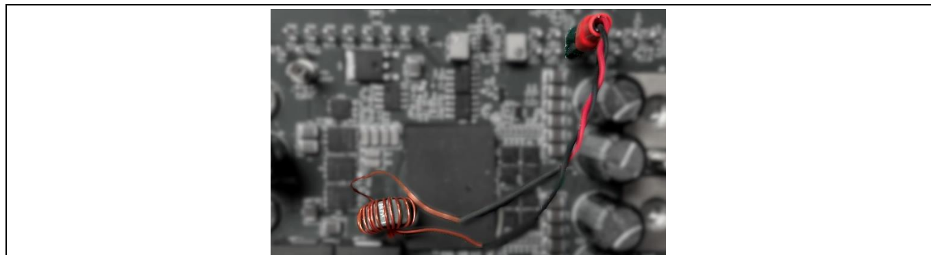
Figure 6 Primary AC current sensing transformer connected to J7
