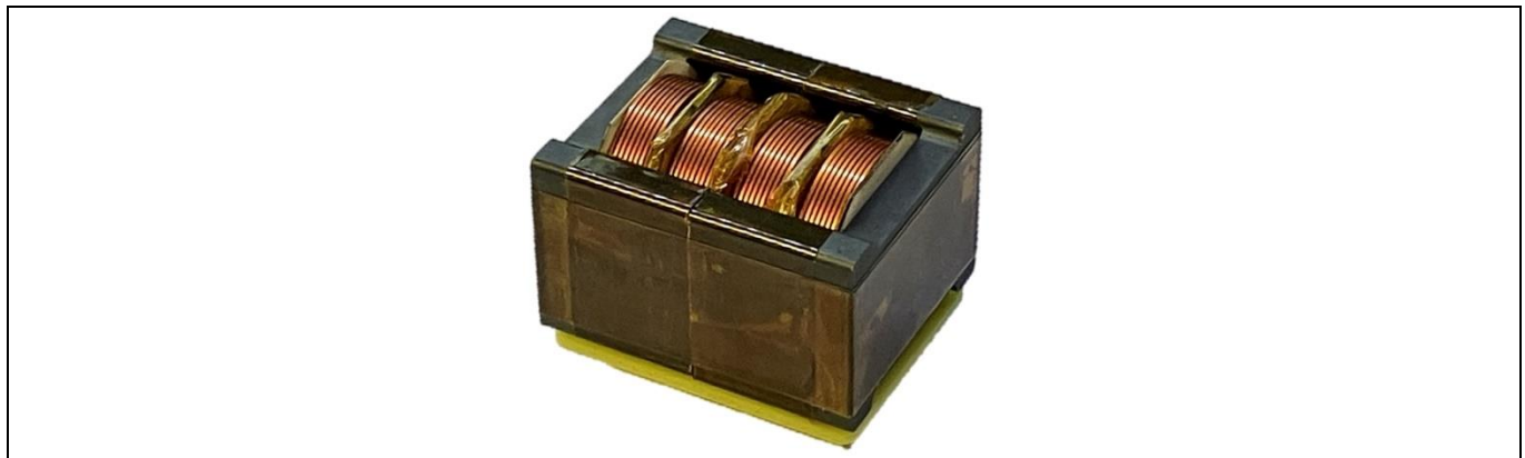
Figure 35 Finished common-mode choke prototype
