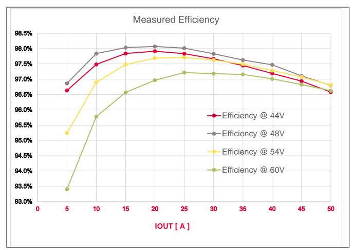
Figure 43 Measured efficiency
