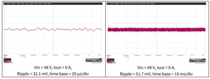
Figure 37 Output ripple at Vin =48 V, lout = 0 A
