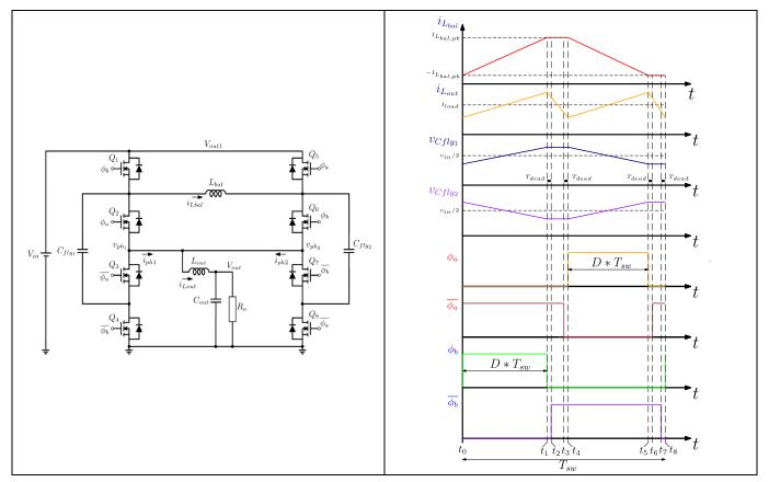
Figure 3 DP-3LFC convertor and main operation waveform with D < 0.5
