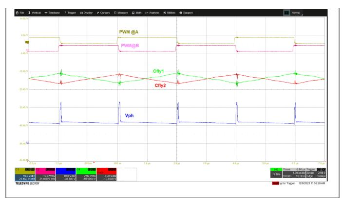
Figure 34 3LFC-DP, basic operation waveforms showing the phase node voltage and the ripple voltage on  $C_{fly1}$  and  $C_{fly2}$  and according to PWM signals at  $V_{in} = 48 \text{ V}$  @ $I_{out} = 40 \text{ A}$ .
