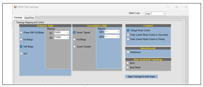
Figure 22 ZSC topology and PWM mapping
