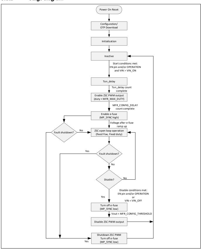
Figure 27 ZSC (loop1) stage diagram
