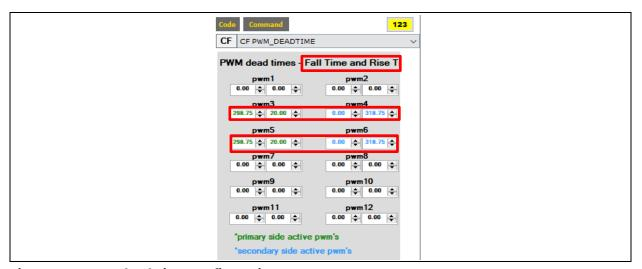
Figure 21 3LFC dead-time configuration
