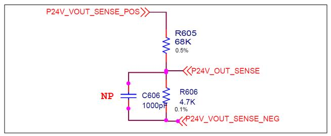
Figure 25 Vmid voltage sensing circuit
