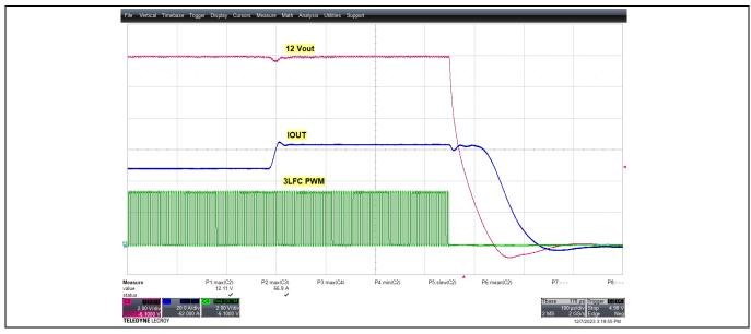
Figure 47 Output OCP waveform at Vin = 48 V, lout = 50 A to overcurrent
