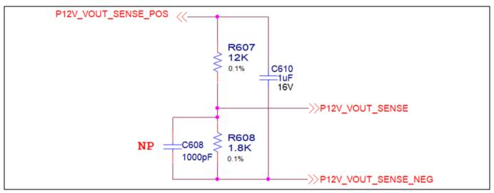
Figure 26 Output voltage sensing circuit
