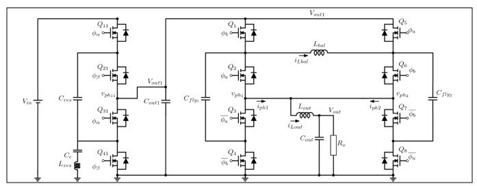
Figure 1 Two-stage ZVS switched capacitor and three-level dual-phase buck converters with balancing inductor (DR-HSC)
