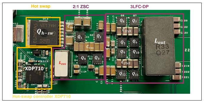
Figure 11 Top-view of the demo board for the regulated 48 V to 12 V DR-HSC converter
