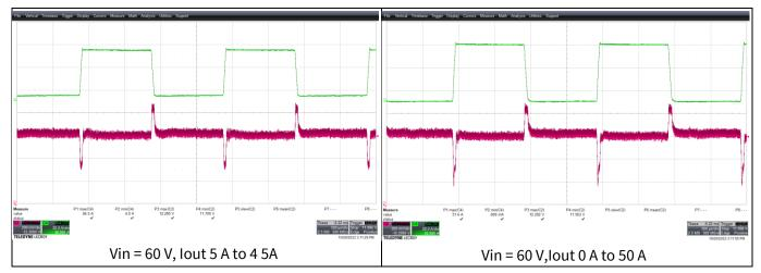
Figure 42 Load transient at Vin = 60 V
