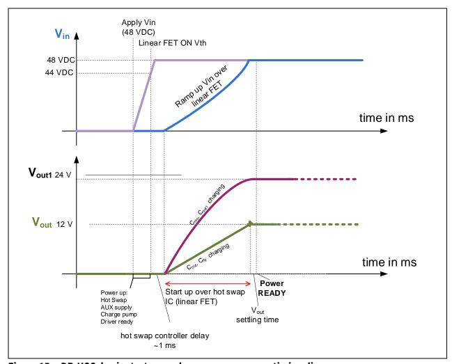
Figure 15 DR-HSC, basic startup, and power up sequence timing diagram
