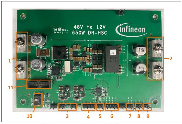
Figure 14 DR-HSC main input and output voltage connection lugs
