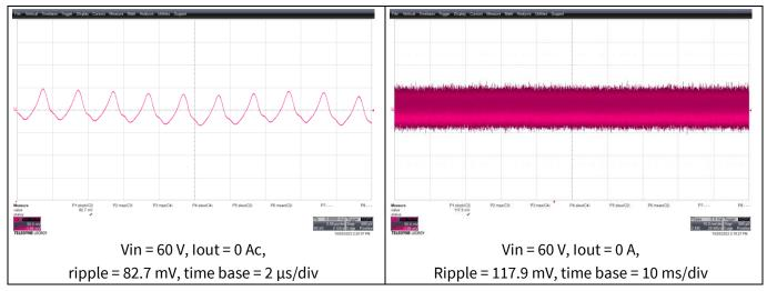
Figure 39 Output ripple at Vin = 60 V, lout = 0 A
