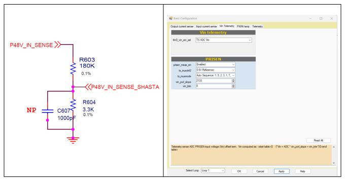
Figure 24 Input voltage sensing by PRISEN pin
