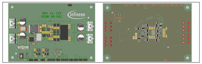
Figure 9 Top and bottom side of the DR-HSC board
