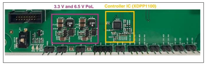
Figure 13 Controller IC and aux power location of the hardware demonstrator
