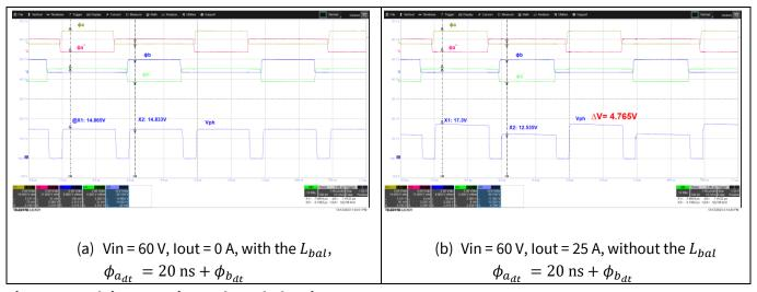
Figure 5 Flying capacitor voltage balancing
