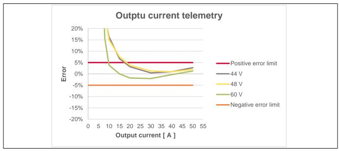
Figure 33 Output current telemetry reading accuracy
