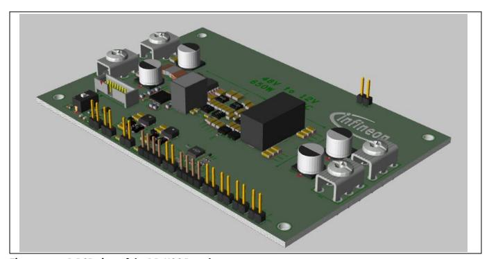
Figure 10 3D PCB view of the DR-HSC Board
