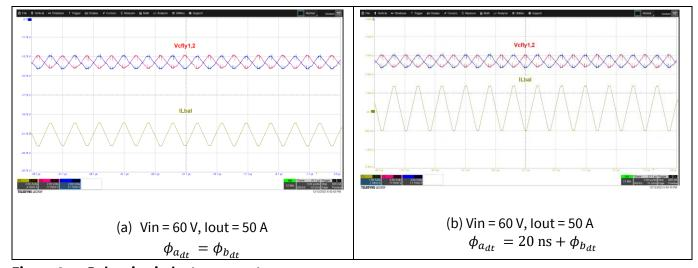
Figure 6 Balancing inductor current
