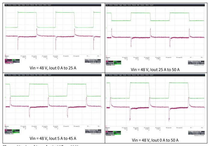
Figure 41 Load transient at Vin = 48 V
