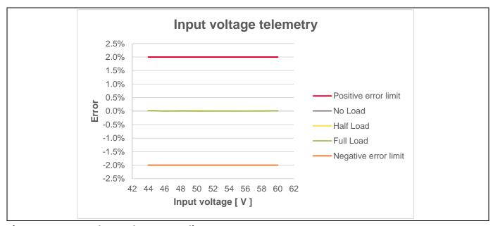
Figure 31 Input voltage telemetry reading accuracy
