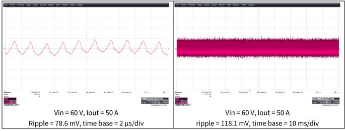
Figure 40 Output ripple at Vin = 60 V, 50 A
