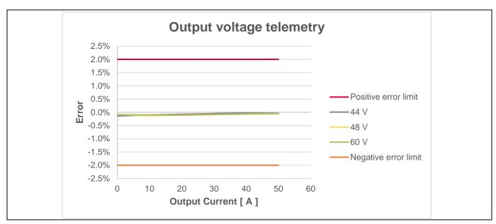
Figure 32 Output voltage telemetry reading accuracy
