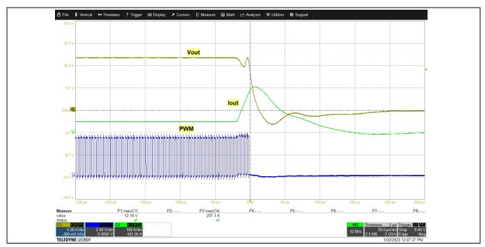
Figure 48 Output short circuit waveform using load bank
