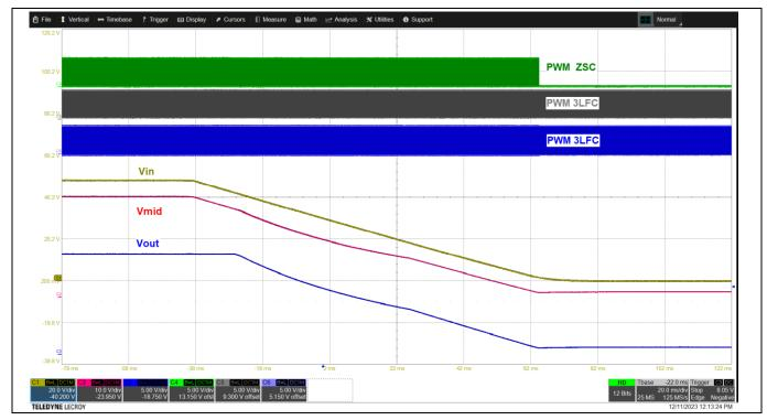
Figure 36 Shutdown behavior at Vin = 48 V, lout = 0 A
