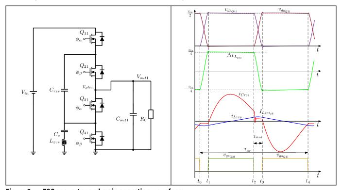
Figure 2 ZSC convertor and main operation waveform
