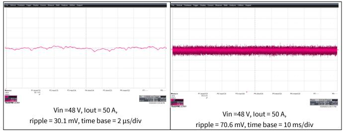
Figure 38 Output ripple at Vin = 48 V, lout = 50 A
