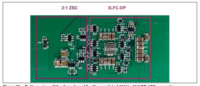
Figure 12 Bottom-view of the demo board for the regulated 48 V to 12 V DR-HSC converter
