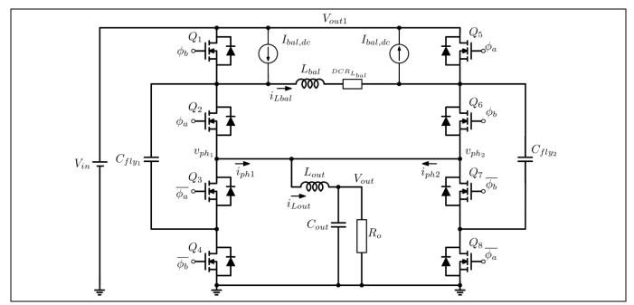
Figure 4 Three-level dual-phase buck converters with equivalent balancing model
