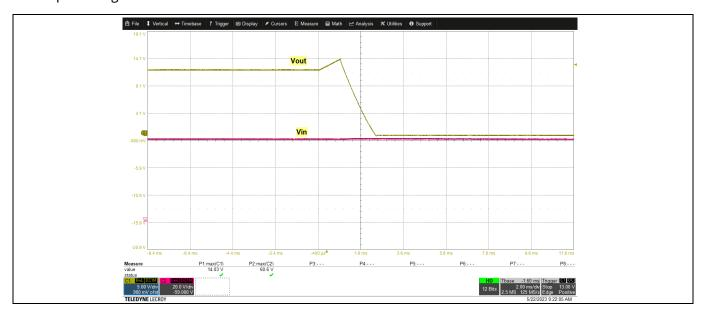
Figure 46 Output OVP waveform at Vin = 60 V, lout = 0 A
