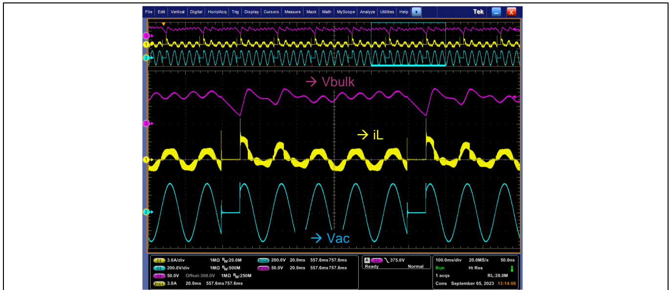
Figure 15 Detail of the 8 th and 9 th repetitions of the 10 ms, 45 degrees LCDO test applied at 230 V – 50 Hz and full load
