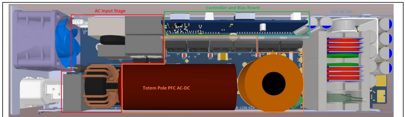
Figure 3 Functional blocks on the PSU board - top view
