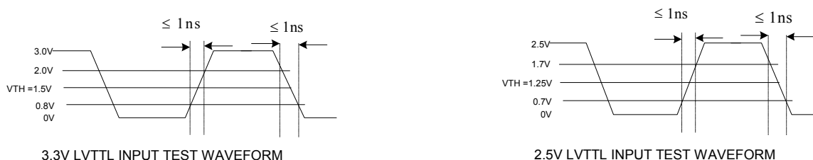
Figure 4. 3.3 V LVTTTL and 2.5 V LVTTTL Input Test Waveforms
