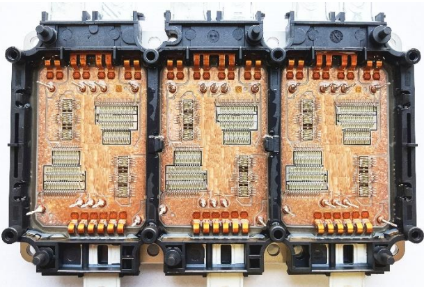
Figure 10: Si/SiC Fusion internal power module layout and signal connections. Each topological switch comprises 3x20 mm 2 SiC MOSFET in parallel with 160 mm 2 IGBT and 60 mm 2 Diode dies.
