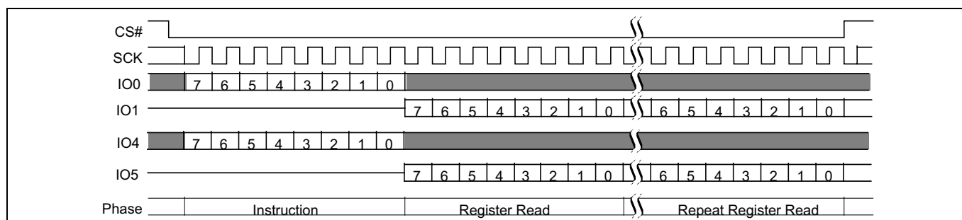
Figure 38 Read Bank Register (BRRD 16h) command
