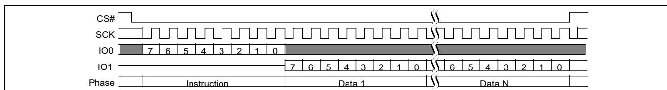
Figure 32 Read Identification (RDID 9Fh) command sequence
