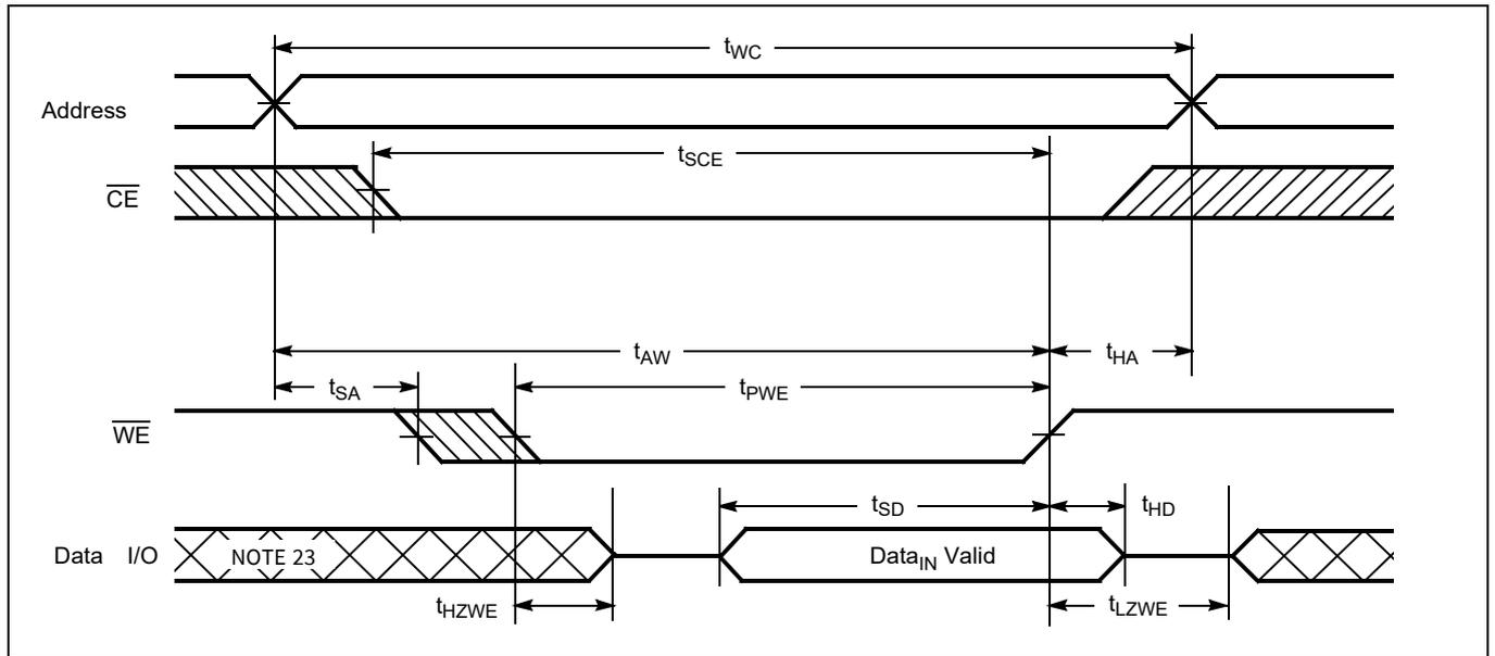
Figure 8 Write cycle No. 3 ( $\overline{WE}$  Controlled,  $\overline{OE}$  LOW)
