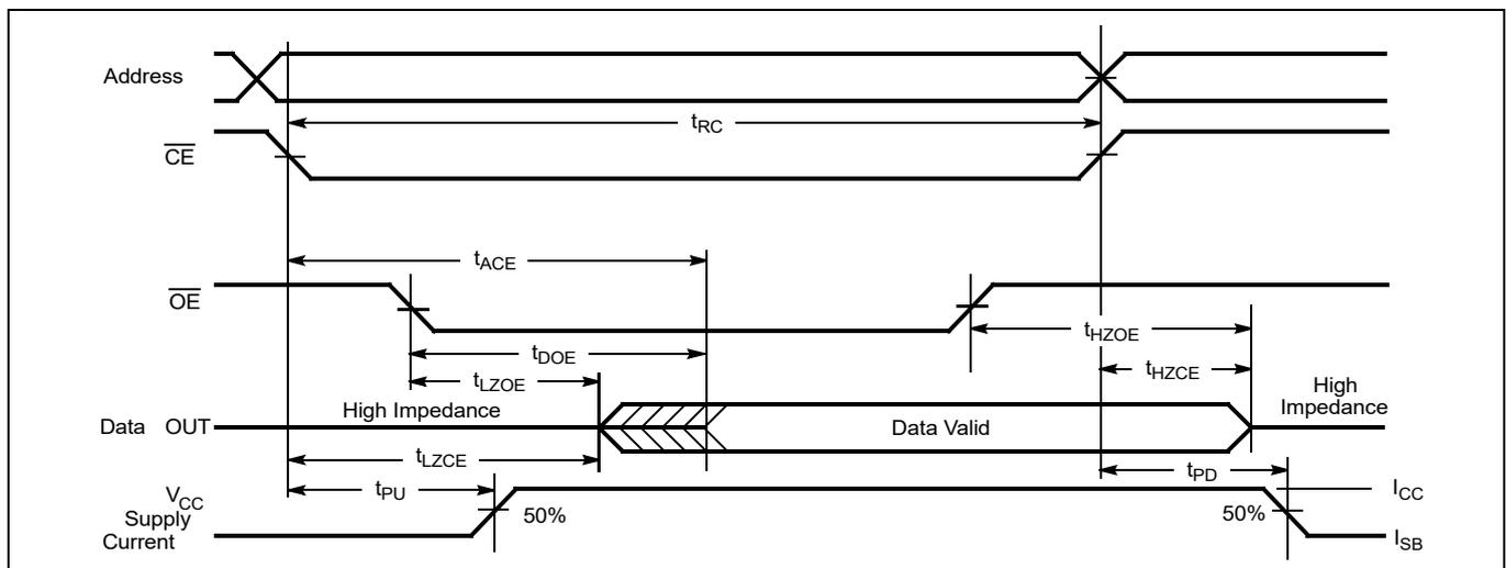
Figure 5 Read cycle No. 2 ( $\overline{OE}$  Controlled,  $\overline{WE}$  HIGH)<sup>[18, 19]</sup>
