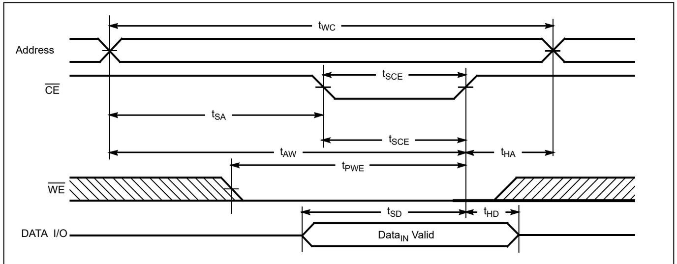
Figure 6 Write cycle No. 1 ( $\overline{CE}$  Controlled)<sup>[20, 21]</sup>
