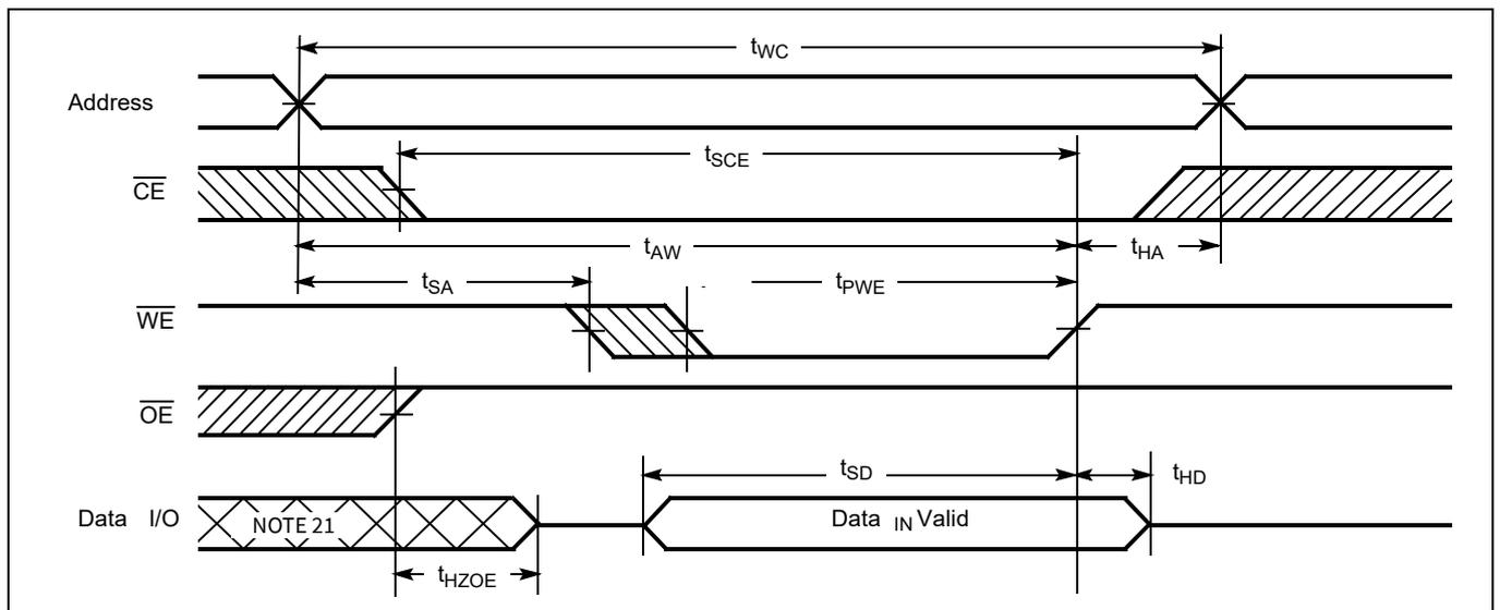
Figure 7 Write cycle No. 2 ( $\overline{WE}$  Controlled,  $\overline{OE}$  HIGH)<sup>[20, 21, 22]</sup>
