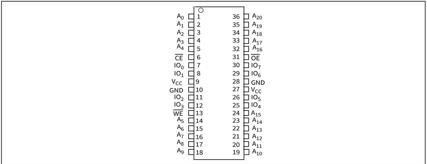
Figure 1 36-pin ceramic flat package pinout (top view) <sup>[3]</sup>
