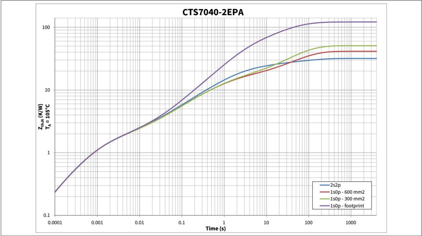
Figure 9 Typical Thermal Impedance. PCB setup according Chapter 4.4.1
