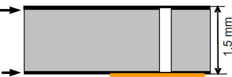
Cross Section (JEDEC 1s0p) with Cooling Area
