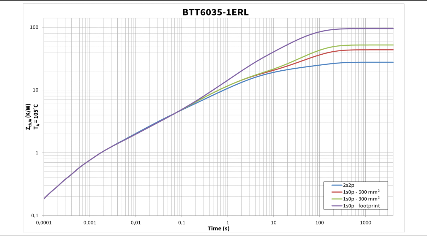
Figure 7 Typical Thermal Impedance. 2s2p set-up according Figure 5
