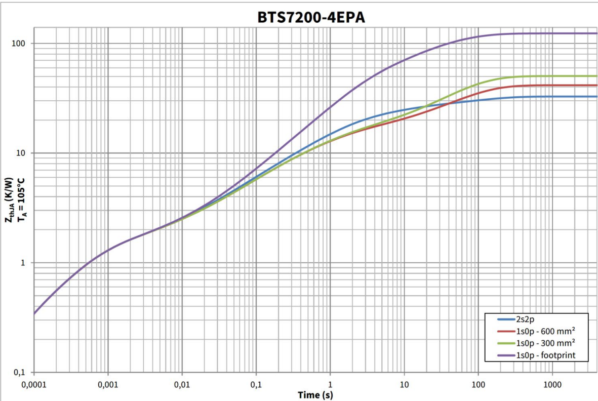
Figure 9 Typical Thermal Impedance. PCB setup according Chapter 4.4.1
