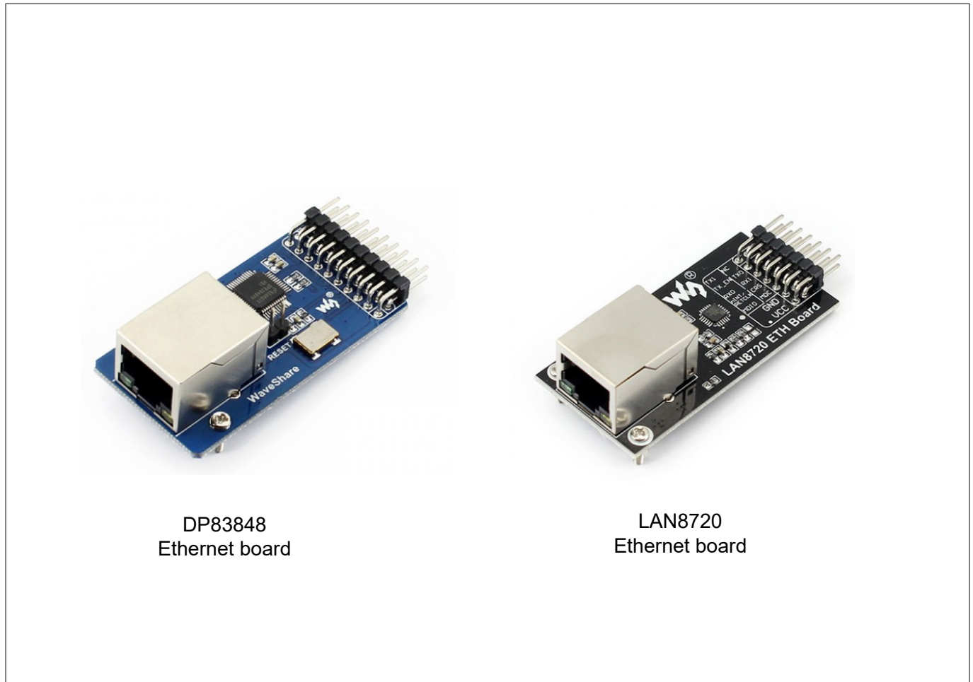
Figure 24 Different Ethernet shields supported by the TRAVEO™ T2G Cluster 4M Lite Kit
