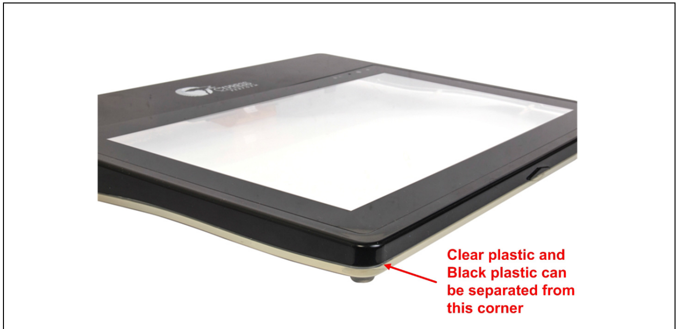
Figure 22 Bottom corner of the case to open plastic case
