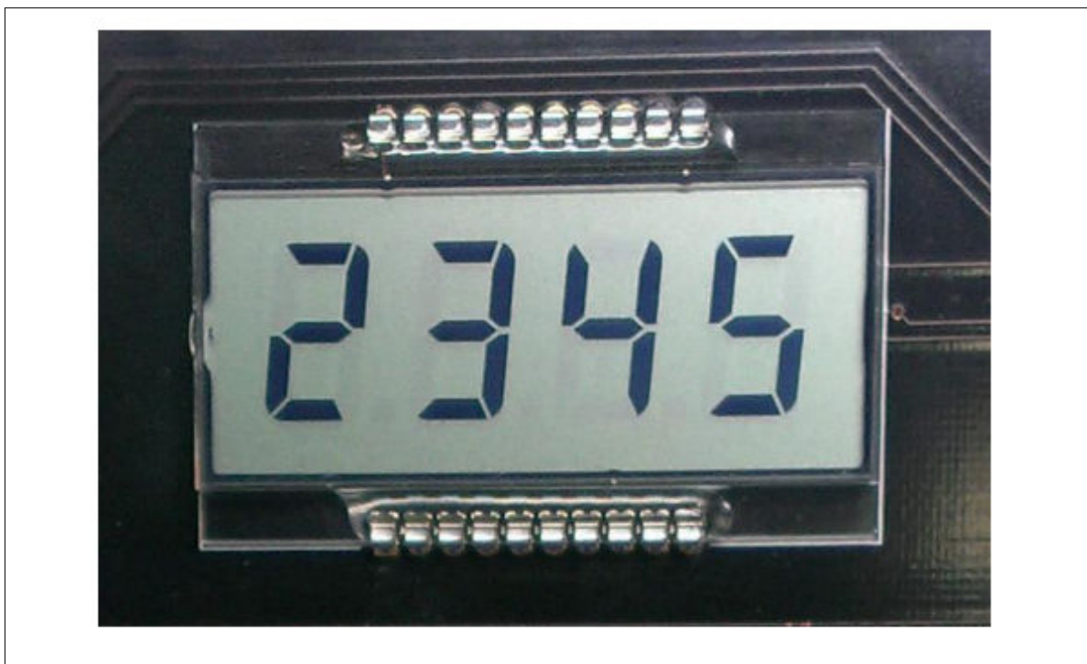
Figure 17 LCD display module scrolling numbers
