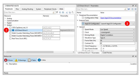
After you have created Segment LCD configuration for your application and used the Device Configurator to configure the Common and Segment signals, you can then use the Segment LCD Configurator without the Device Configurator on subsequent updates.
