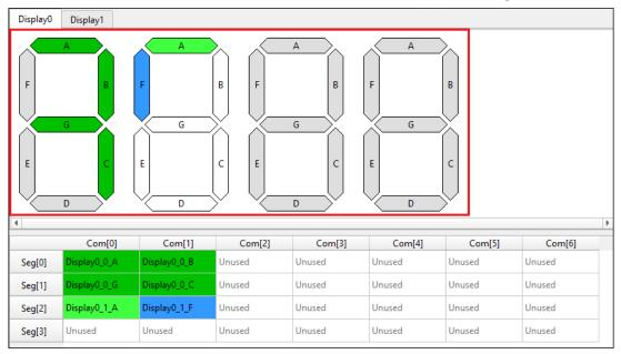
A display symbol contains a set of pixels named A, B, C... (or 00, 01, 02 for the matrix display type) by default. The pixel names correspond to cell names in the Mapping table (for a pixel placed on the mapping table). The pixels have colors showing the connectivity status:
