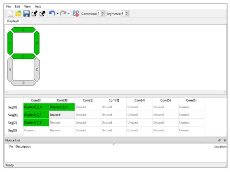
The Segment LCD Configurator GUI contains menus and display view to configure display tabs, and a Notice List to provide indications.
