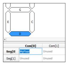
Once the name has been changed, only the first two characters of the pixel name show in the display name. To return a pixel name to its default value, delete the name and press [Enter].
