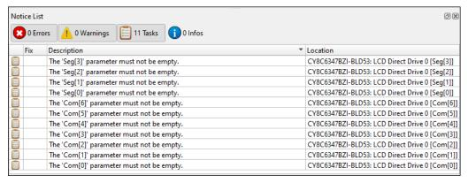
**9.** Double-click one of the task icons to jump to the Parameters pane for the corresponding connection parameter. Click the pull-down menu and select the appropriate signal.
