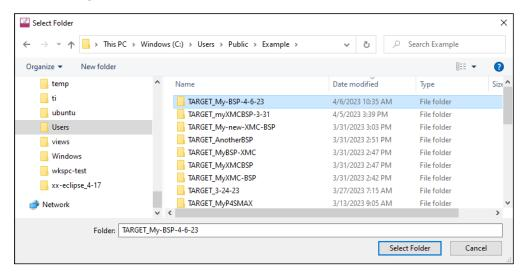
Navigate to and select the appropriate folder containing the BSP to import and click **Select Folder**. The tool checks that the BSP begins with the name "TARGET\_" and that it has a makefile, but it does **not** validate the makefile for correctness. If the selected BSP is correct, it is added to the list with all the other BSPs.
