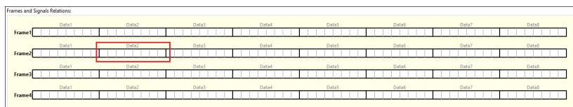
One frame length can be any from 1 to 8 data bytes. Each byte contains eight 1-bit cells: Data1 through Data8. The total number of frames cannot exceed 60. The total size of all frames is limited to 256 bytes.
