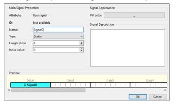
The "Signal Properties" dialog displays if you click the Add button on the toolbar to configure and add a new signal or double-click an already configured and added signal's symbol to edit its configuration.
