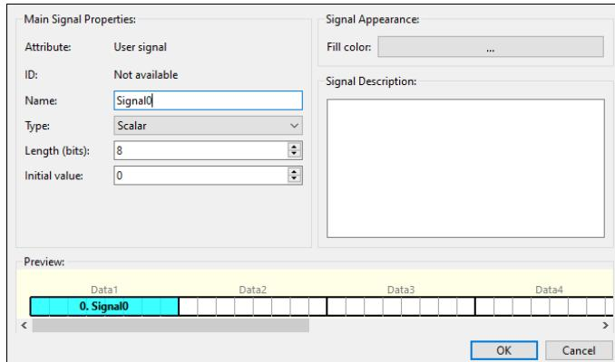
The "Signal Properties" dialog displays if you click the **Add** button on the toolbar to configure and add a new signal or double-click an already configured and added signal's symbol to edit its configuration.
