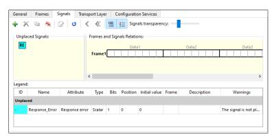
The subtab toolbar and panes – Unplaced Signals, Frames and Signals Relations, Legend – are described in the following sections.
