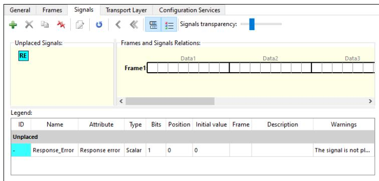
The subtab toolbar and panes – Unplaced Signals, Frames and Signals Relations, Legend – are described in the following sections.
