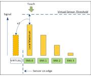
If the Edge correction is enabled, the algorithm adds a virtual neighbor sensor to correct the deviation in the reported position. The Virtual sensor signal is defined by the Virtual sensor threshold:
