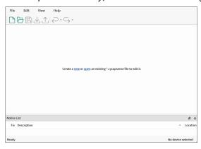
You must open an existing \*.cycapsense file or create a new one for the application in which you want to configure CAPSENSE™, and it must be in the same directory as the design.modus file.
