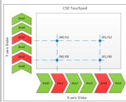
But, if this feature is enabled, the CSD touchpad can report up to two touches, mainly to be used in conjunction with two-finger gestures where real and ghost touches do not need to be fully differentiated. It is available for the CSD touchpad only when the Centroid type is configured to 5x5.
