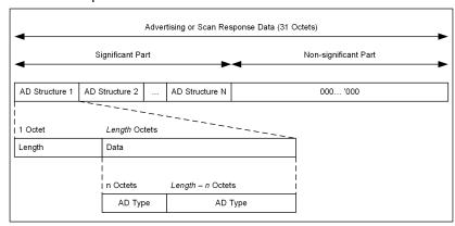
A data packet can contain a number of AD structures. Each of these structures is composed of the following parameters:
