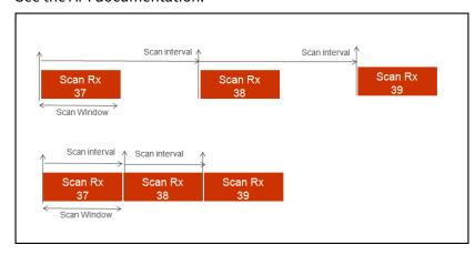
Fast scan parameters – This connection type results in a faster connection between the GATT Client and Server devices than it is possible using normal connection.
