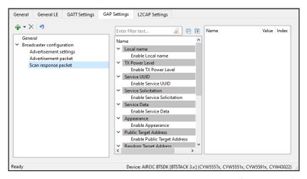
The **Scan response packet** structure is the same as of the **Advertisement packet**. See Advertisement / Scan response packet data settings under GAP Settings tab Advertisement packet for information on configuring the **Scan response packet**.
