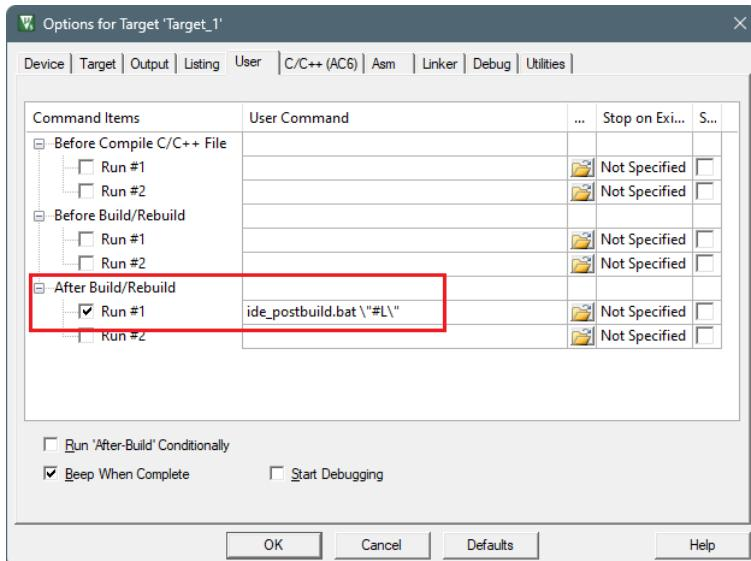
3. Next, build the application. The post-build script will handle the signing process for you. All other configuration steps are the same as those in [Device with default policy](#). After a successful build, you can program the device and start a debugging session. For more details on device provisioning and hex file signing, refer [Application Note AN240106 - Getting started with PSOC™ Control C3 security](#).
