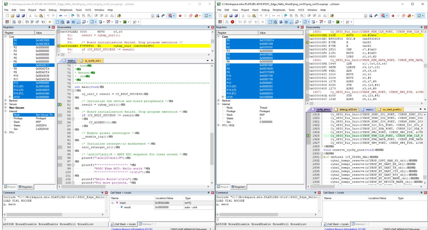
The left side of the screen shows a µVision IDE instance attached to the CM33 core. The right side shows the CM55 core has not started yet. Once the `Cy_SysEnableCM55()` function on the CM33 core has been executed, the CM55 will start executing its application. You can step through the code by switching back and forth between the two µVision IDE instances.
