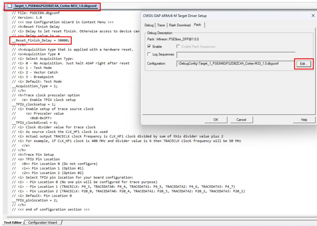
By default, the Test Mode acquisition is applied after XRES.
