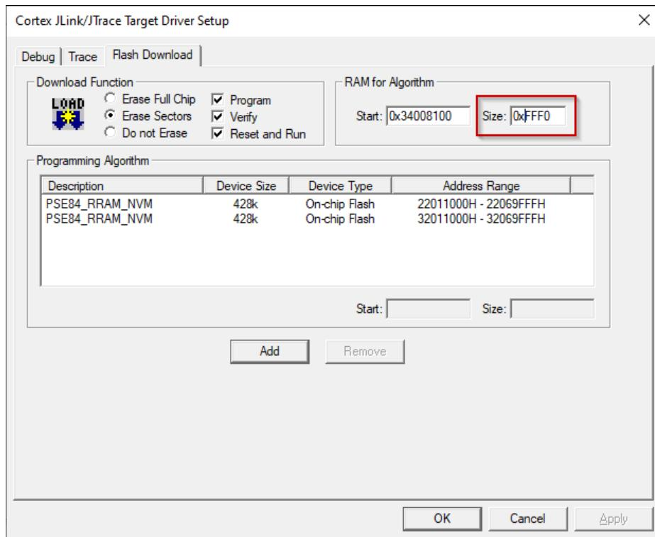
8. For either driver, if any application (secure CM33, non-secure CM33, or CM55) should be programmed to external memory, two additional instances of flashloaders with name PSE84\_SMIF need to be added using the **Add** button.
