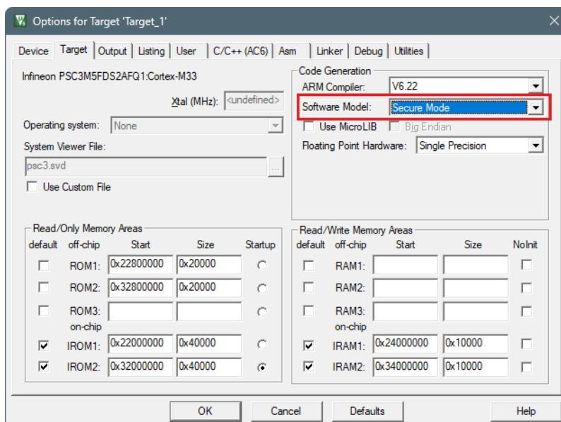
Save the application and select **Project > Build Target** to build it. The Output should display the progress, ending with text similar to this:
