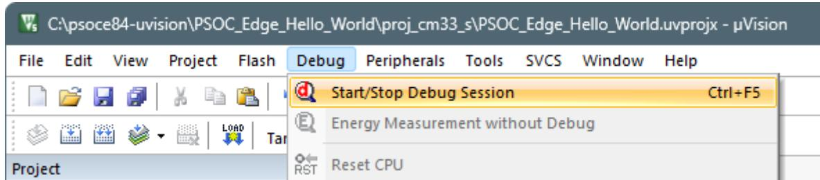
This will reset the target and halt execution at the beginning of the `main()` function of the CM33 project.
