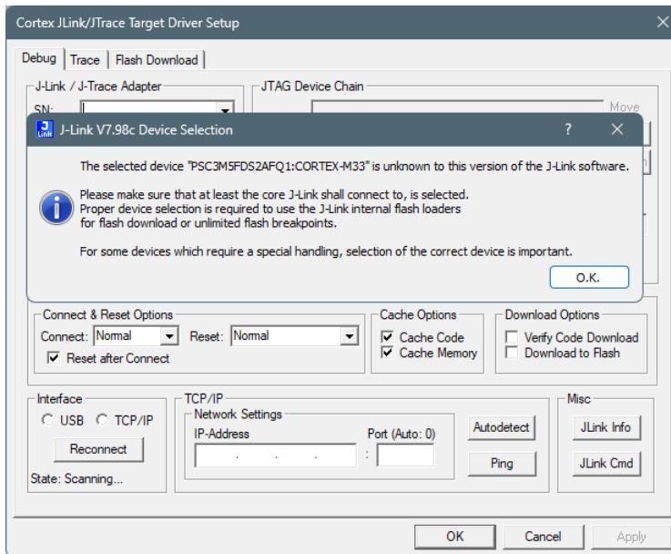
4. Select the appropriate device in the Target device settings and click **OK**.
