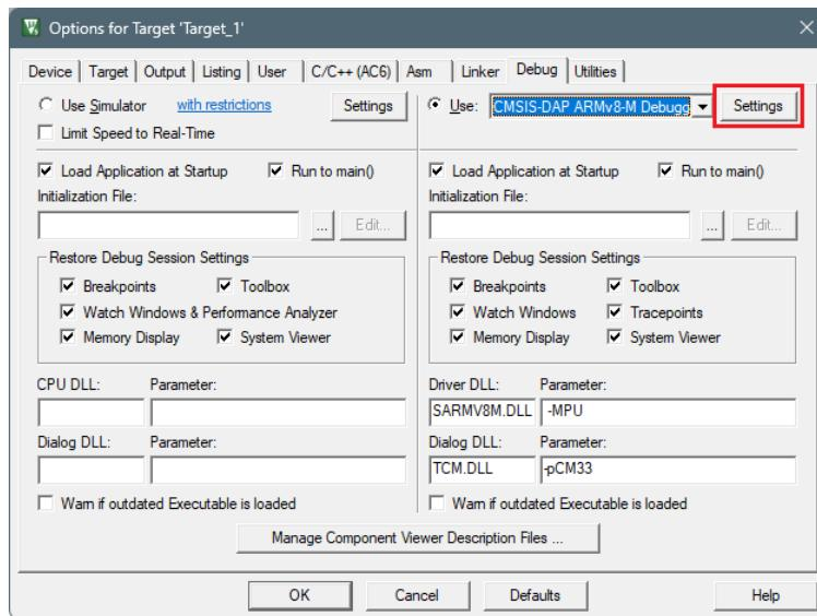
4. On the Target Driver Setup dialog on the **Debug** tab, select the following:
