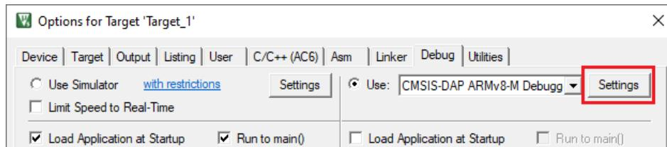
5. Select the **Debug** tab, and choose applicable connection options, the configuration settings are different for CMSIS-DAP and J-Link. Refer to the following sections for the applicable options:
