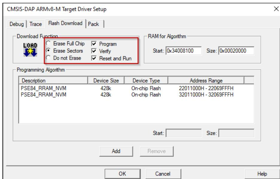
7. For J-Link, ensure the RAM size for the algorithm is set to 0xFFFF0.
