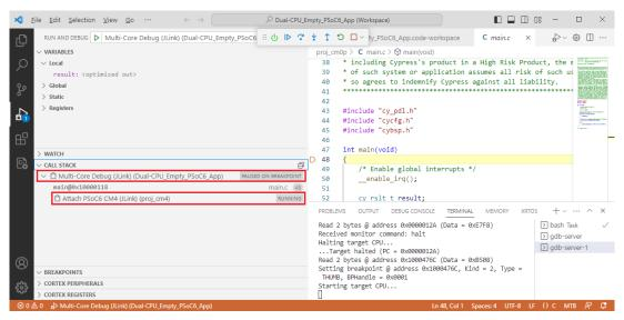
Once a session has started, the CM0+ core is halted at the beginning of main(), while the CM4 core is spinning in an endless loop in boot code, waiting for start. It will start and halt at main() as soon as the application running on the CM0+ executes the Cy SysEnableCM4() function.
