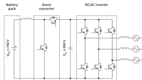
Figure 4: A typical converter topology for utility-scale ESS
