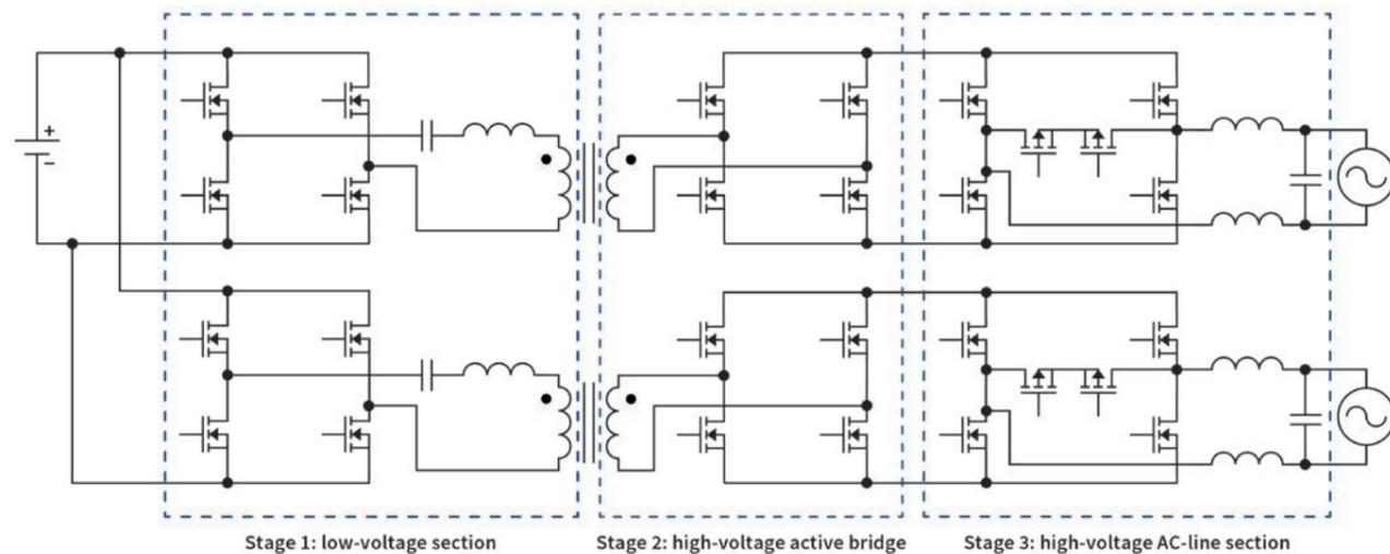
Figure 2: A possible converter topology for residential ESS
