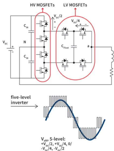
Figure 3: 5-level flying capacitor active neutral point clamp inverter basic schematic
