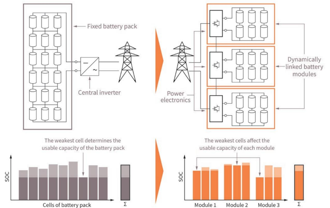
Figure 5: Battery-charge flexibility in cascaded modular multilevel ESS
