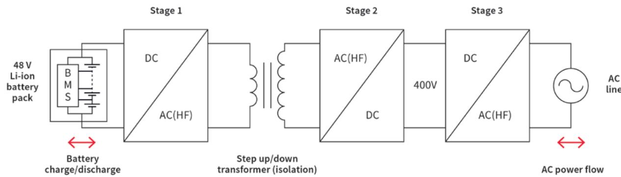
Figure 1: Basic block diagram for a residential energy storage system
