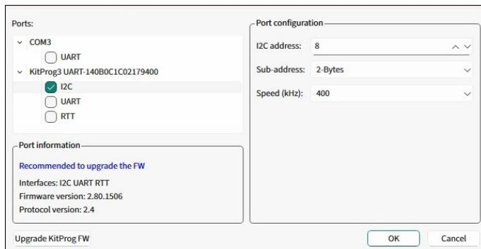
To establish the **I2C** communication between the Tuner and target device, configure the Tuner communication parameters to match the parameters of the device EzI2C settings.
