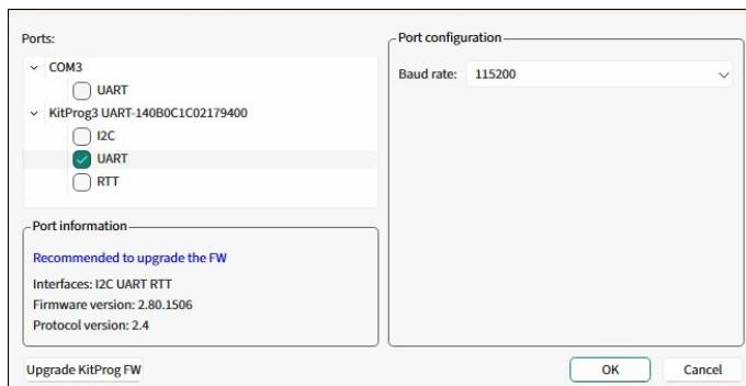
To establish the UART communication between the Tuner and target device, configure the Tuner communication parameters to match the parameters of the device UART settings.
