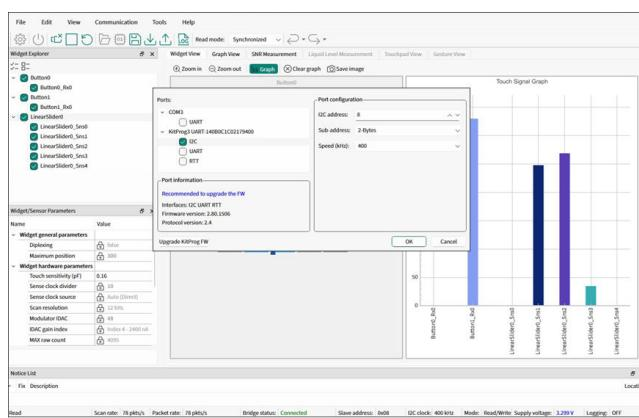
**Note:** *For MiniProg, first, power the device – click the **Tuner Communication Setup** button to select the communication interface, use the **Power** button to select and apply the power supply, and proceed with **Connect**.*
