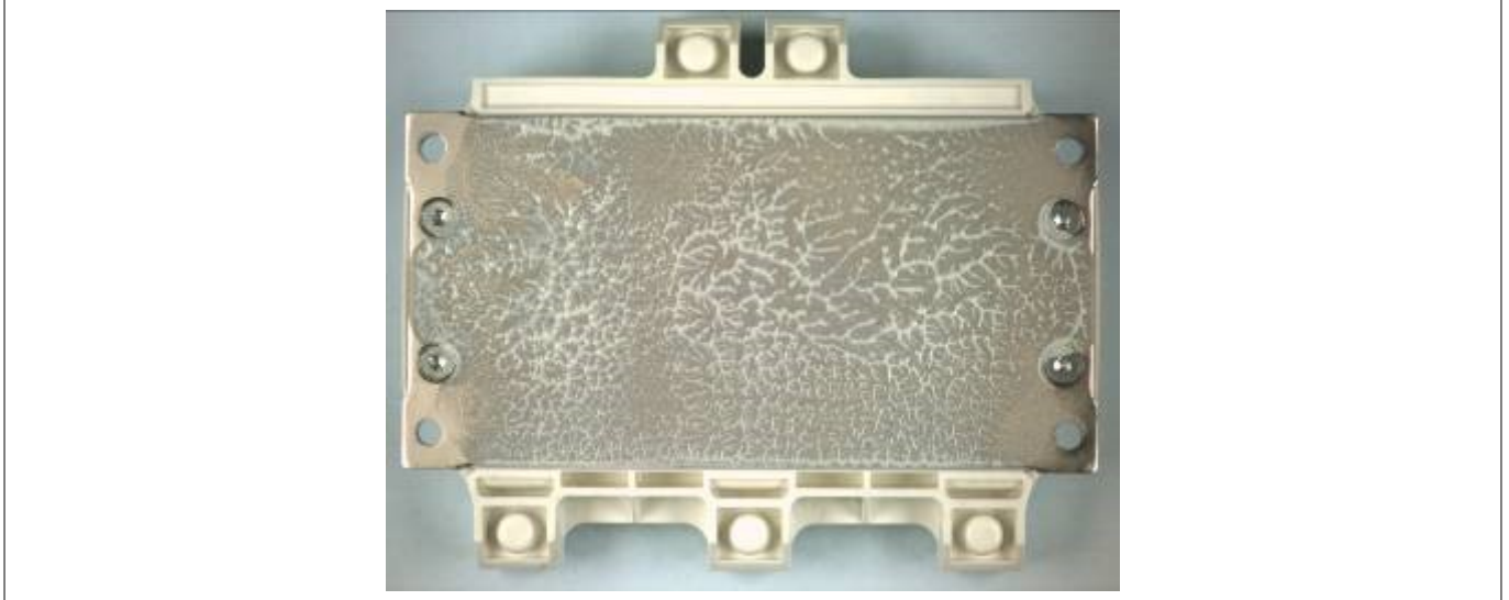
Figure 5 Print image of HybridPACK™ 1 disassembled with a branch-like thermal compound structure
