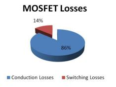
Figure 3.2: MOSFET losses in the application
