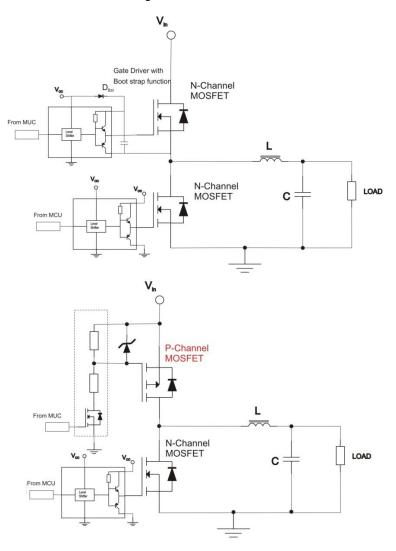
Figure 3.3: Buck converter circuit
