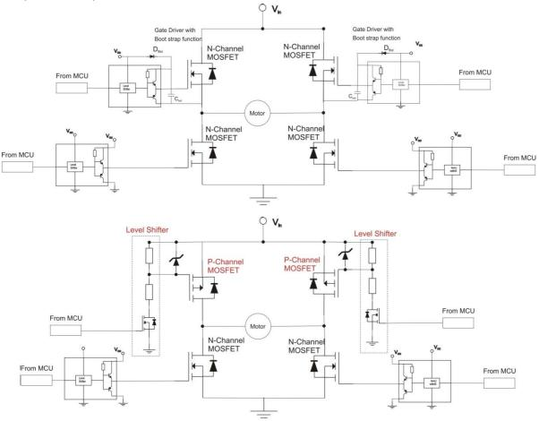
Figure 3.1: Low-Voltage drive application circuit
