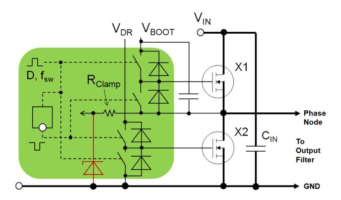
Figure 7 Clamped voltage protection for phase node by (red) clamp structure, voltage drops across R<sub>Clamp</sub>
