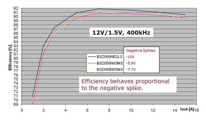
Figure 4 Example of how switching speed impacts the efficiency, RDSON of all parts is about identical and its impact is minor as it can be observed by comparison of BSZ050N03MS (5.0 mΩ @ VGS=10 V) and BSZ058N03MS (5.8 mΩ @ VGS=10 V). BSZ060NE2LS has 6.0 mΩ @ V
