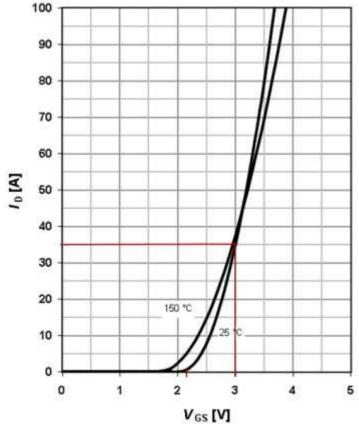
Figure 6 Transfer characteristic of the BSZ060NE2LS (Tj as parameter)
