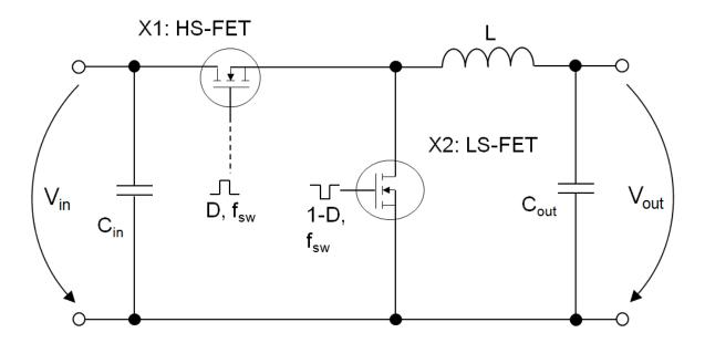
Figure 1 Standard buck-converter with synchronous rectification
