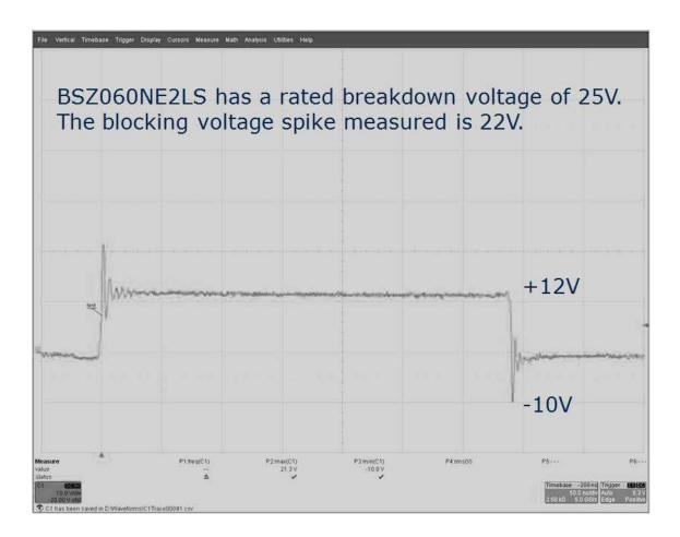
Figure 5 Measured spike
