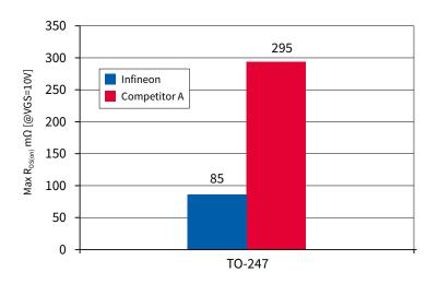
Infineon's new CoolMOS<sup>TM</sup> best-in-class TO-247 part has more than 71% lower  $R_{\rm DS(on)}$  than the nearest competitor
