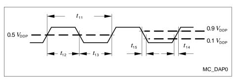
Figure 21 Test Clock Timing (DAP0)
