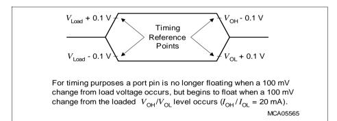
Figure 16 Floating Waveforms
