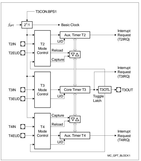
Figure 7 Block Diagram of GPT1
