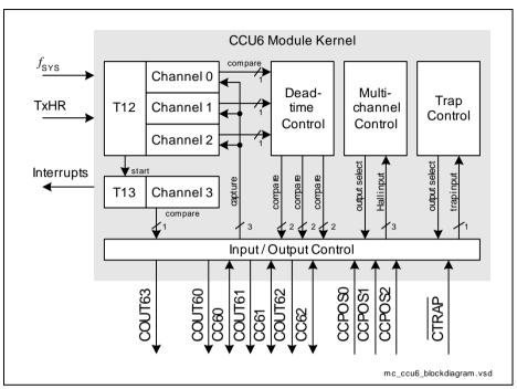
Figure 6 CCU6 Block Diagram
