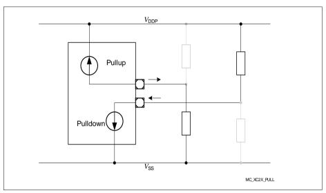
Figure 11 Pullup/Pulldown Current Definition
