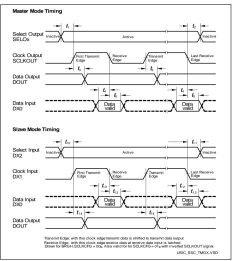
Figure 20 USIC - SSC Master/Slave Mode Timing
