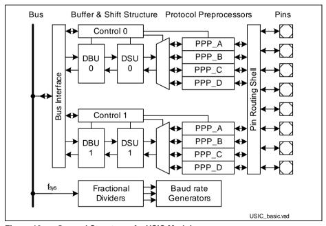
Figure 10 General Structure of a USIC Module
