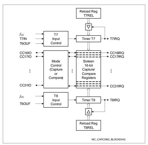
Figure 5 CAPCOM Unit Block Diagram
