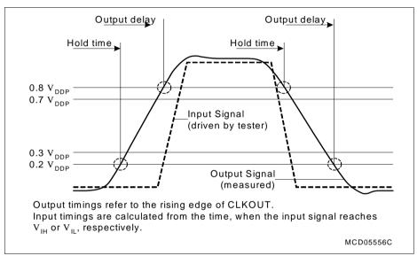
Figure 15 Input Output Waveforms
