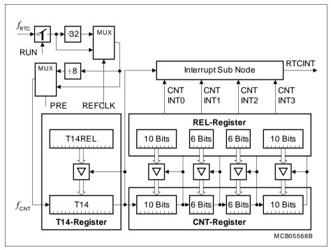
Figure 9 RTC Block Diagram
