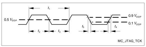
Figure 24 Test Clock Timing (TCK)
