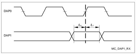
Figure 22 DAP Timing Host to Device
