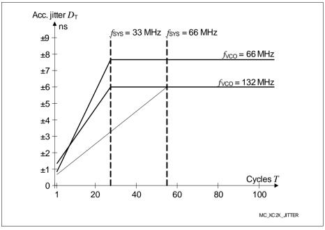
Figure 18 Approximated Accumulated PLL Jitter
