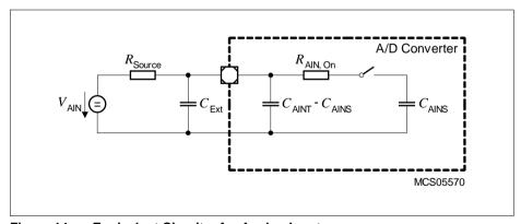
Figure 14 Equivalent Circuitry for Analog Inputs
