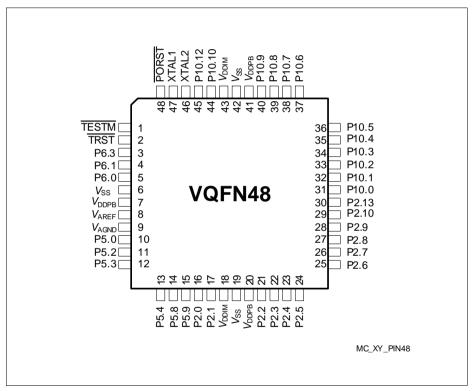
Figure 2 XC2220U Pin Configuration (top view)
