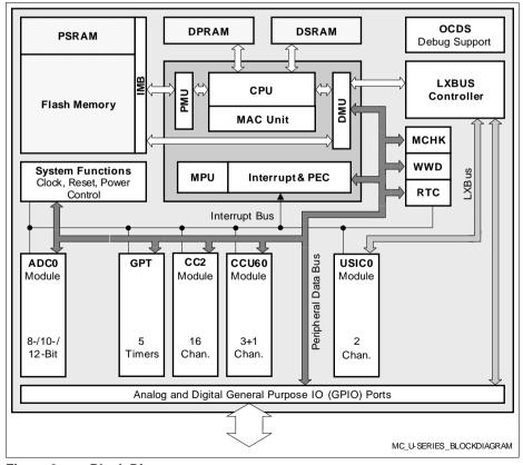
Figure 3 Block Diagram
