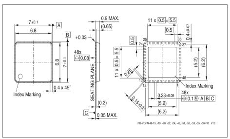
Figure 26 PG-VQFN-48-54 (Plastic Green Thin Quad Flat Package)
