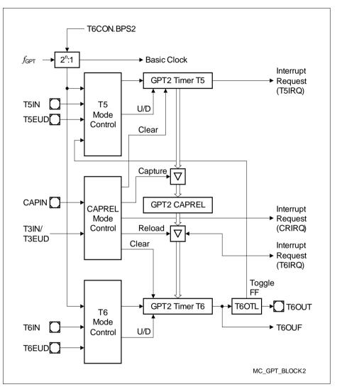
Figure 8 Block Diagram of GPT2
