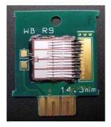
(a) Cu-clip IGBT. (b). Wire-bonded IGBT Fig. 5 Top views of IGBTs packaged in Cu-clip (a) and wirebond (b).
