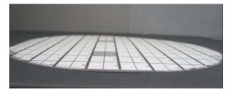
Fig. 4 Wafer with warpage less than 1 mm.
