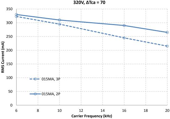
**Figure 6:** Maximum Sinusoidal Phase Current vs. PWM Switching Frequency Sinusoidal Modulation, V<sup>+</sup>=320V, PF=0.98
