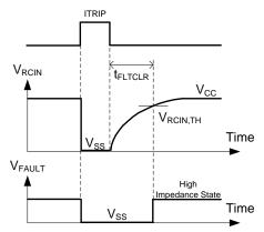
Figure 5: RCIN and FLT pin waveforms
