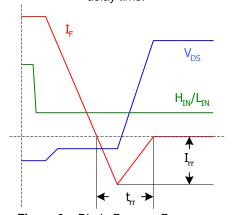
Figure 2c: Diode Reverse Recovery.
