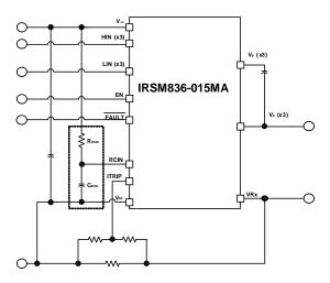
Figure 4b: Programming the fault clear timer
