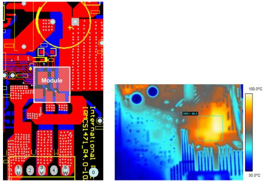
Figure 7: PCB layout example and corresponding thermal image (10kHz, 3P, 1oz, ΔTca=70°C, V+ = 320V, Iu = 295mArms)
