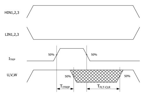
Figure 3: I<sub>TRIP</sub> Timing Waveform
