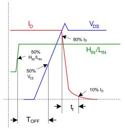
Figure 2b: Input to Output propagation turn-off delay time.
