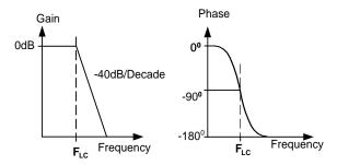
Figure 26: Gain and Phase of LC filter
