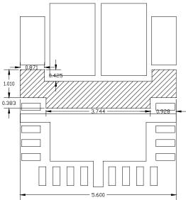
Figure 44: PCB Pad Sizes Detail 2 (Dimensions in mm)
