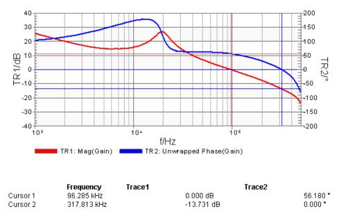
Figure 40: CH1 Bode Plot with 6A load, CH2 disabled. Fo = 96.3 kHz, Phase Margin = 56.2 Degrees
