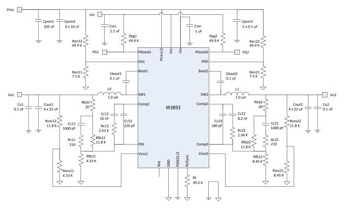
Figure 30: Application circuit for a 12V to 1.8V and 1.2V, 4A Point of Load Converter using external 5V VCC
