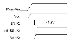
Figure 5: Recommended startup for Normal operation
