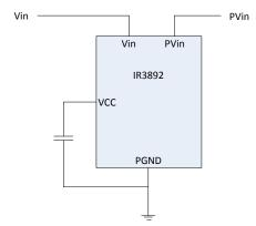
Figure 13: Internally Biased Configuration
