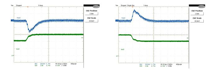
Figure 39: Vout2 Transient Response, 4.2A to 6A step at 2.5A/μSec CH1:Vout1, CH2=Vout2, CH4:Iout2
