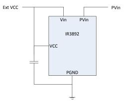
Figure 15: Externally Biased Configuration
