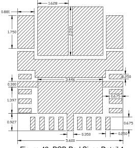
Figure 43: PCB Pad Sizes Detail 1 (Dimensions in mm)
