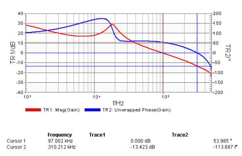
Figure 41: CH2 Bode Plot with 6A load, CH1 disabled. Fo = 97 kHz, Phase Margin = 54 Degrees
