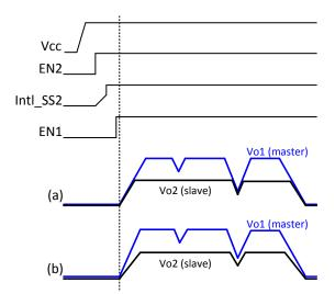
Figure 19: Typical waveforms for sequencing mode of operation: (a) simultaneous, (b) ratiometric
