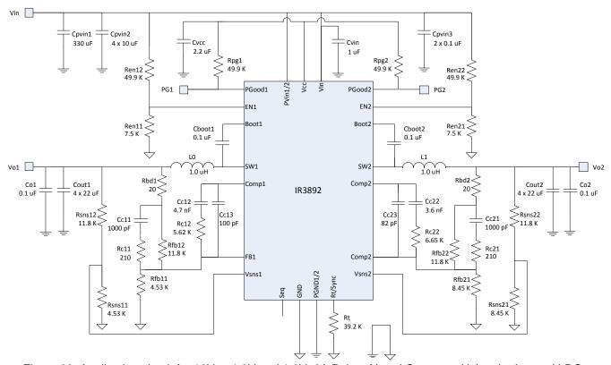
Figure 29: Application circuit for 12V to 1.8V and 1.2V, 6A Point of Load Converter Using the Internal LDO
