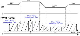
Figure 12: Timing diagram for Feed Forward (F.F.)
