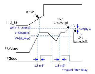
Figure 16: Timing Diagram for Output Sequence
