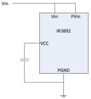
Figure 14: Internally Biased Single Rail Configuration
