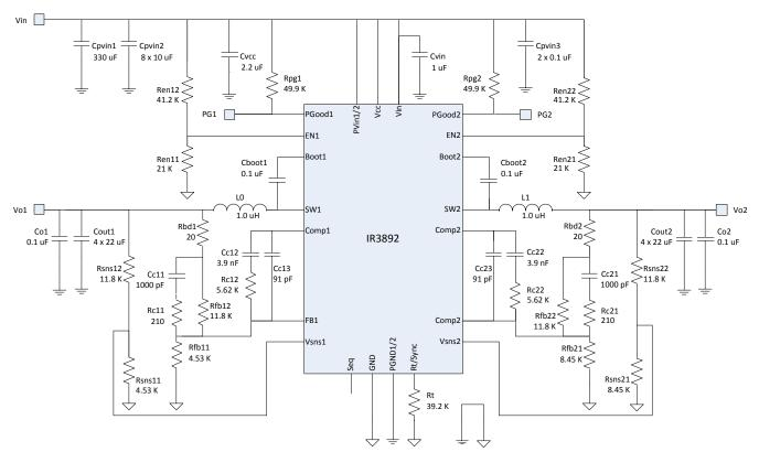
Figure 31: Application circuit for a 5V to 1.8V and 1.2V, 4A Point of Load Converter
