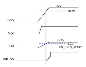
Figure 4: Normal Startup: IR3892 Channel starts when PVin reaches 10.2V by connecting EN to PVin using a resistor divider.
