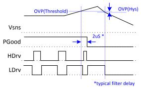
Figure 20: Timing diagram for OVP
