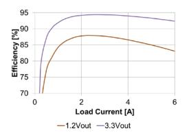
Figure 2: Efficiency [Vin=12V, Fsw=600kHz]
