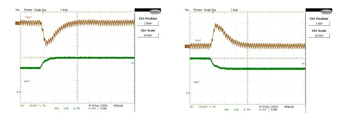
Figure 38: Vout1 Transient Response, 4.2A to 6A step at 2.5A/μSec CH1:Vout1, CH2=Vout2, CH4:Iout1
