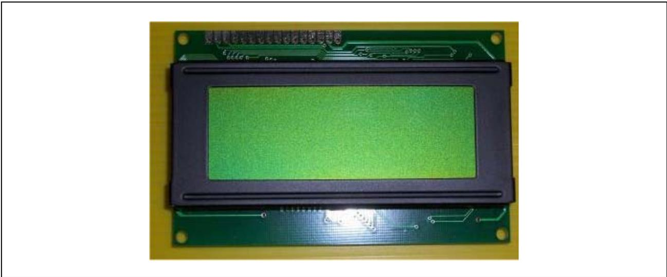
**Figure 1 The TM204 display module**
