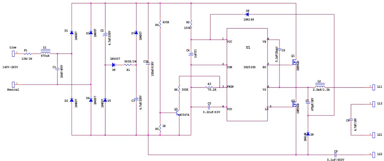
Fig. 4: Electrical Circuit - 14W CFL Ballast
