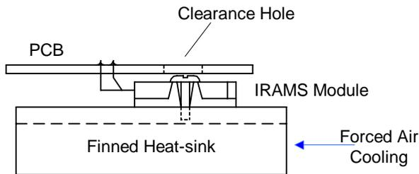
Figure 2: 90° Lead-Form Mounting
