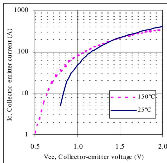
**Figure 6.** Typical output characteristic of the GA200SA60S
