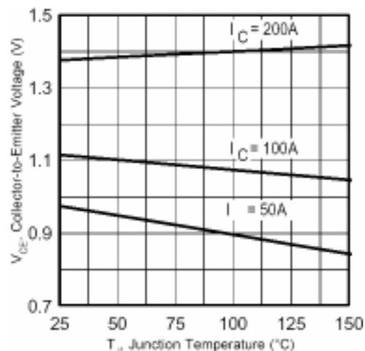
**Figure 5.**  $V_{CE(on)}$  voltage drop vs. temperature in the GA100TS60SQ
