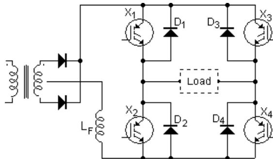
**Figure 1.** Simplified circuit of the Full-Bridge output Inverter.
