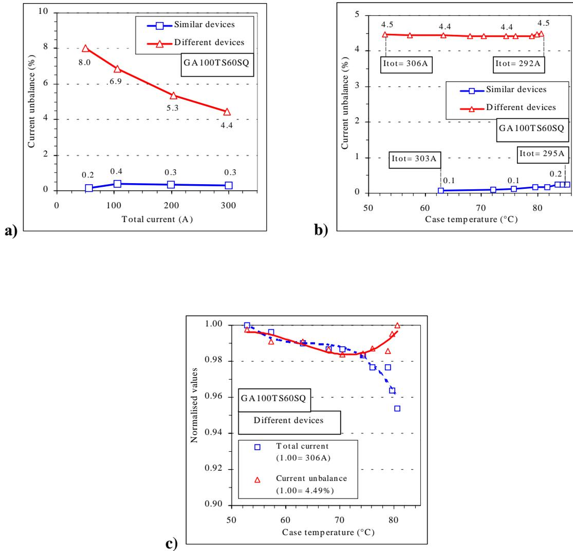
**Figures 8a, b and c.** Operation of two GA100TS60SQ connected in parallel to a DC power supply
