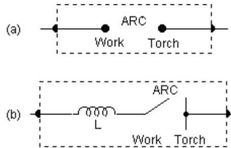
Figure 2. Models of the load: (a) basic and (b) more accurate
