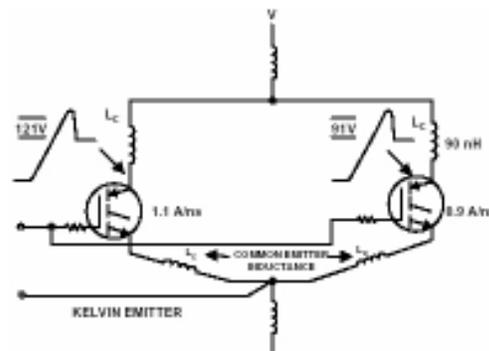
**Figure 10.** Parallel connection of two IGBT and example of difference in transient voltage
