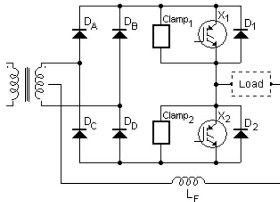
**Figure 4.** Simplified circuit of the Half-Bridge output inverter
