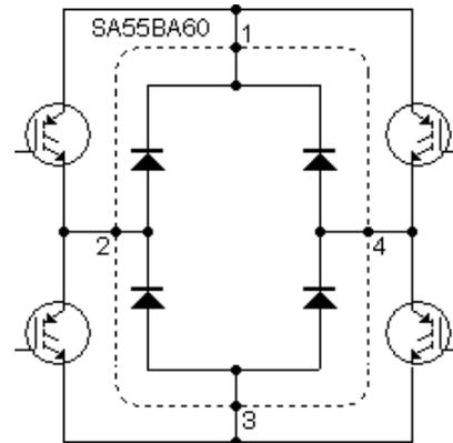
**Figure 3.** Application and pinout of SA55BA60 in “H-Bridge” inverters (load not shown)
