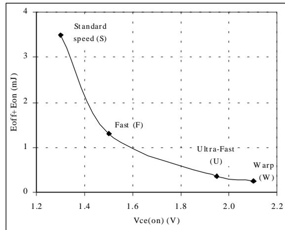
Figure 7. Example of  $E_{tot}$  vs.  $V_{CE(on)}$  trend
