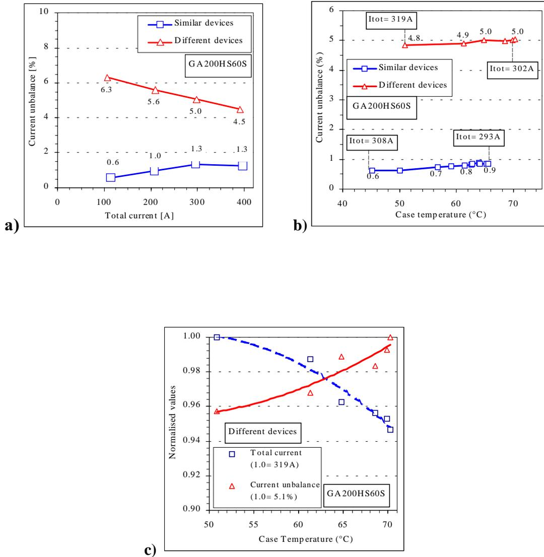
Figures 9a, b and c. Operation of two GA200HS60S connected in parallel to a DC power supply
